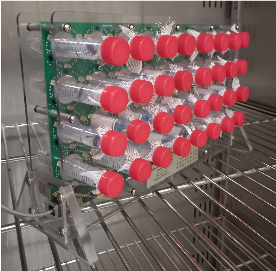
Figure 2. One of the activity monitors used in the experiments. The activity monitor has 32 cells, and each cell can take 15-ml (dimensions: 17 mm O.D., 120 mm length) falcon tube with single honeybee in it.
