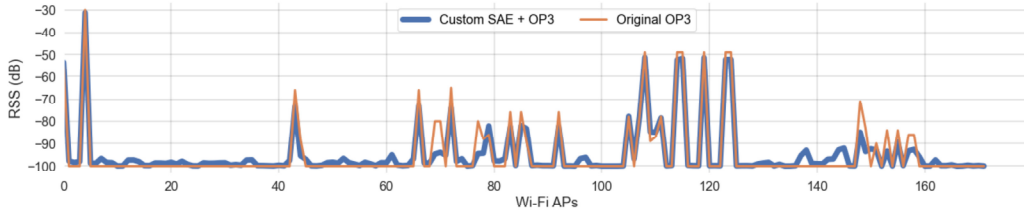
Fig. 10. Comparison of original fingerprint and augmented fingerprint using custom SAE on Device: OP3.
