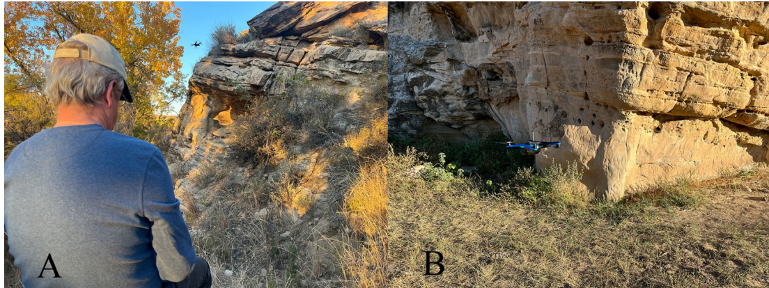
Figure 6. Demonstrations of the sUAS obstacle avoidance capabilities. (A): The Skydio 2+ drone flying between a stand of trees and a cliff. (B): Drone collecting data 30 cm above ground.
