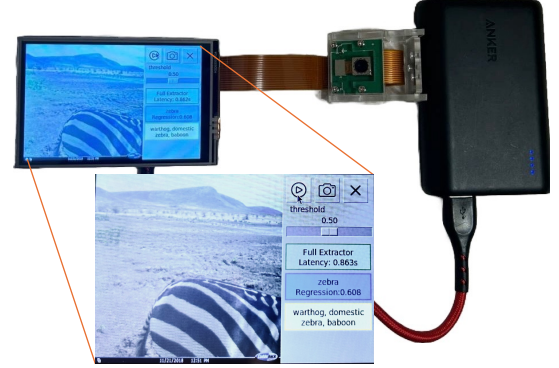
Figure 9: Raspberry Pi Zero W with a camera (mounted on the Raspberry Pi board), LCD display, and a power bank.
