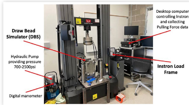
FIGURE 2 The laboratory testing setup: the sheet metal strip is pulled in between the flat inserts clamped by horizontal hydraulic press.
