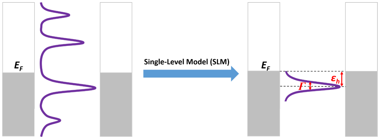
Figure 2. A simplified electronic structure of the molecular junction (right) along with the key parameters \varepsilon_h and \Gamma , obtained from the actual DOS (left) under the assumptions of the SLM.
