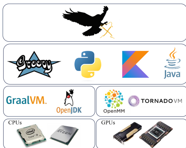
FIG. 1. An overview of Force Field X. The second row shows languages that are compatible with FFX. The third row represents the platforms that execute FFX on CPU cores on the left and coprocessors on the right. The final row indicates the CPU and GPU hardware that FFX can perform calculations on.
