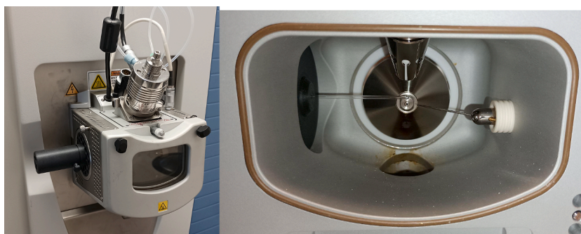
Fig. 12. left. IonMax source housing with APCI source and OpenASAP system installed and mounted on the Q Exactive HF-X. right. View of the MS inlet and source components showing the capillary in the OpenASAP system positioned between the APCI source and MS inlet.
