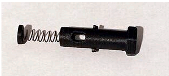
Fig. 9. Probe button, spring, and spacer after before final insertion into the probe body.
