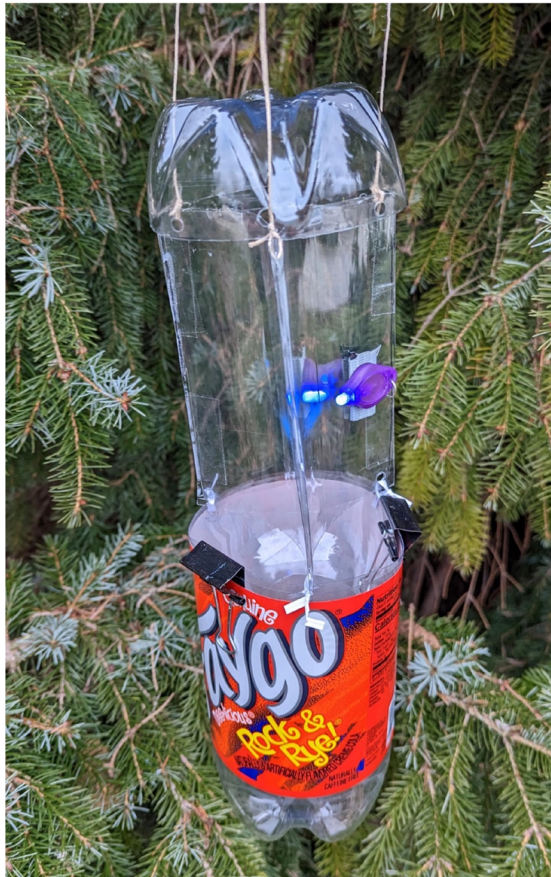
FIGURE 1: Moth trap built using instructions in “Building a simple moth trap” [available in Supplemental Materials ]. Shown with small keychain UV LED light turned on and ready to attract moths.
