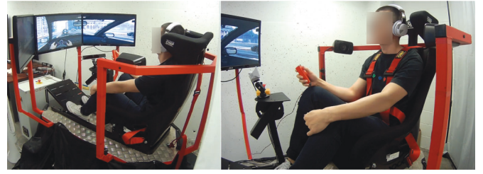
Fig. 2: The high-fidelity driving simulator used in this study.
