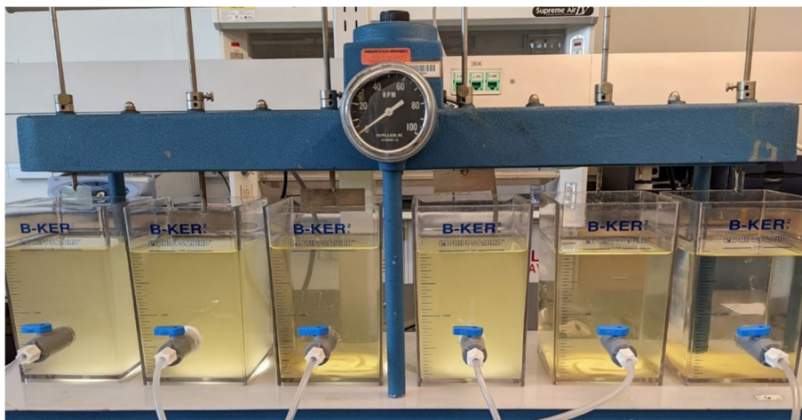
Fig. 2 A photograph showing the results of a typical jar test completed in the physical laboratory mode. The leftmost jar is the control, with chemical dosage increasing to the right. Clearer water is desired
