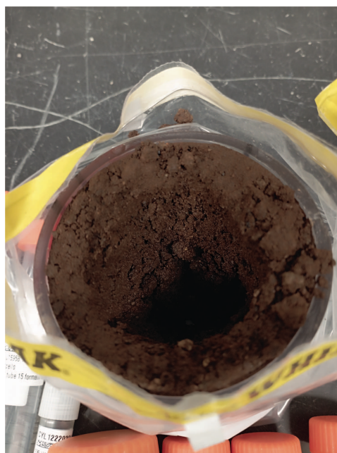
Figure F36. Whole-round sample after subsampling of interior for microbiology, Expedition 398.
