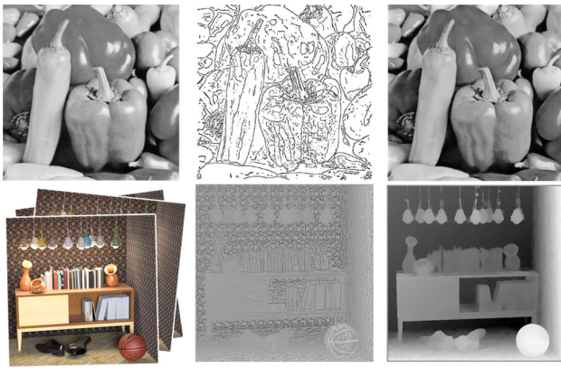
Fig. 1 Top : Elder showed that a representation of image edges including position, brightness and contrast, gradient, and blur scale is complete as it lets us reconstruct the image via a diffusion process with low error. Left to right : Original image, edge locations, reconstructed image; reproduced from Elder (1999). Bottom : We show that a similar approach is possible for multi-view images and provides a complete representation for scene geometry via depth
