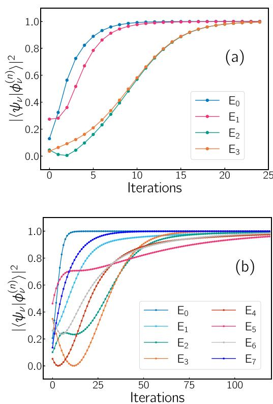
**Figure 1.** Evolution of the projection of the states  $|\psi_\nu^{(n)}\rangle$  on the exact eigenstates  $|\psi_\nu\rangle$  as a function of the iteration  $n$  for (a) 2-qubit and (b) 3-qubit random Hamiltonians in equation (12).
