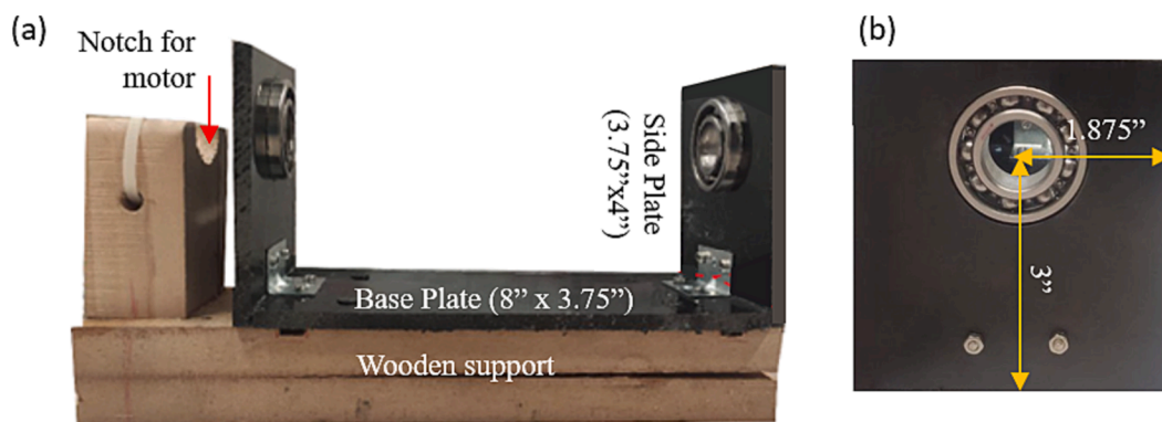
Fig. 5. Components of the frame, which include (a) base Polypropylene frame mounted on a wooden support, (b) the side plate showing the pressure-fitted ball bearing.
