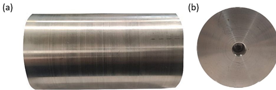
Fig. 6. Components of the drum, which include (a) the front view of the Aluminium drum after smoothing to the required diameter, and (b) side view of the drum showing the internal threading at the center.
