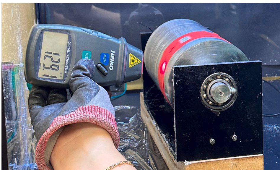
Fig. 24. Using Tachometer to measure rotations per minute on rotating drum.
