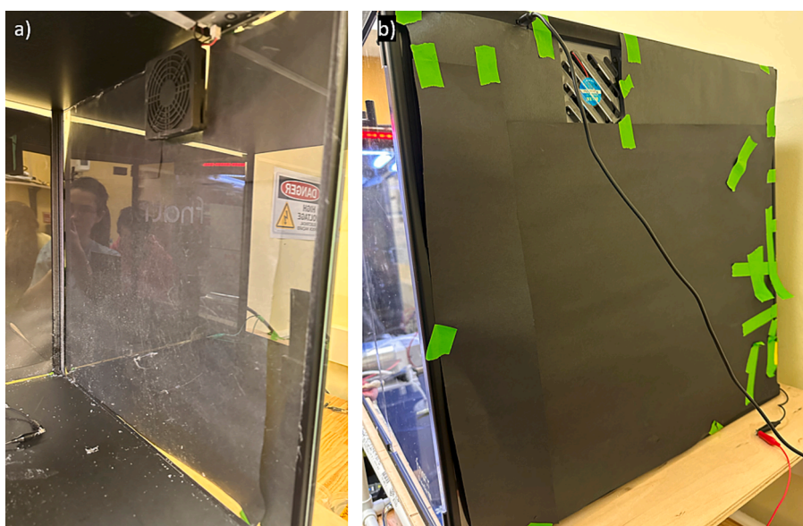
Fig. 18. Environmental chamber covered in black construction paper a) interior view, and b) exterior view.
