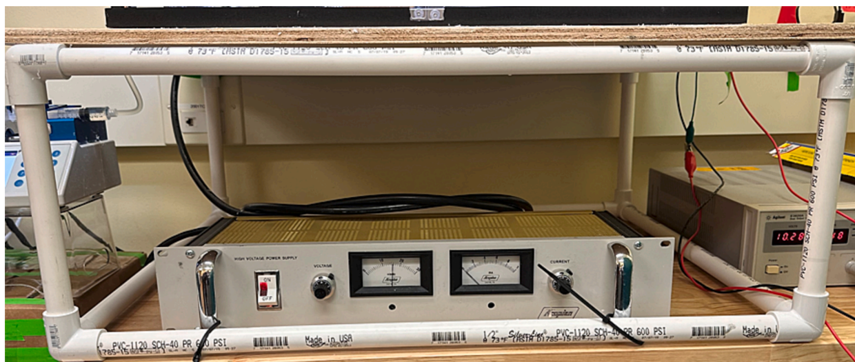
Fig. 16. PVC frame with plywood board to serve as stand, with high voltage power source below and low voltage power source to the right.
