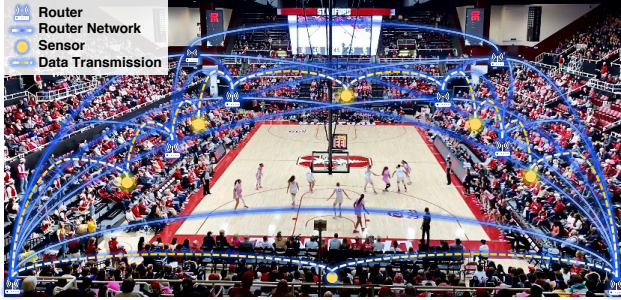
Figure 9: Sensor network of GameVibes . Sensor data are transmitted wirelessly through routers via Wi-Fi connections in the stadium.
