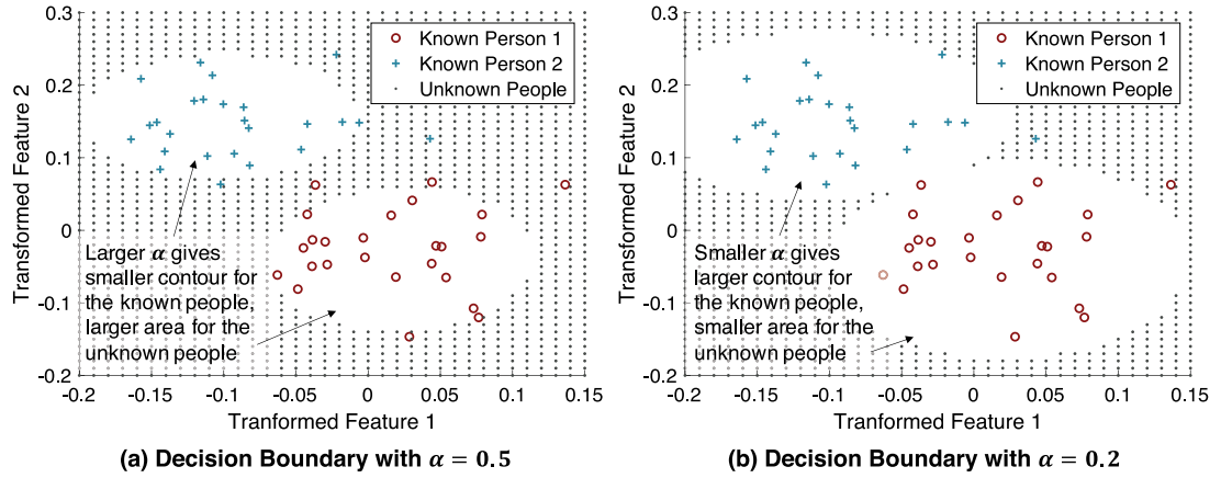
Fig. 9. Decision boundary changes with the hyperparameter \alpha : a larger \alpha means the incoming footsteps are more likely to belong to an unknown person.
