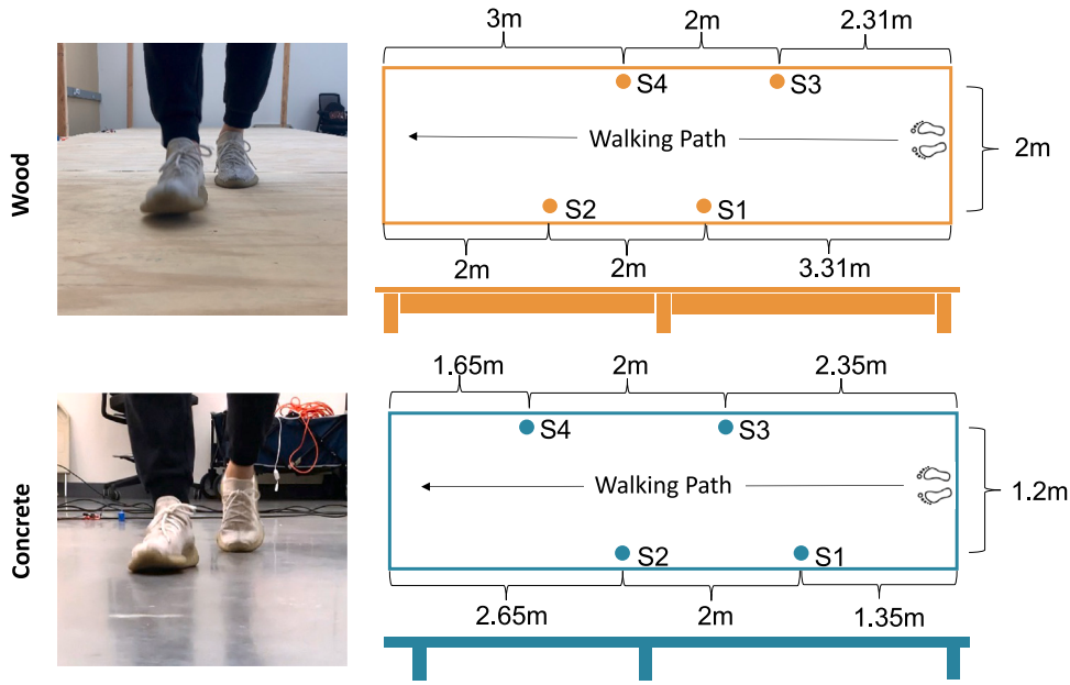
Fig. 10. Walking experiment for evaluation. The experiments were conducted in a real-world setting with human subjects (right). The sensor layout, walking paths, and the cross-sectional structural layout of the wooden structure (top) and the concrete structure (bottom) are shown in the diagram. The floor dimensions are marked in the diagram.
