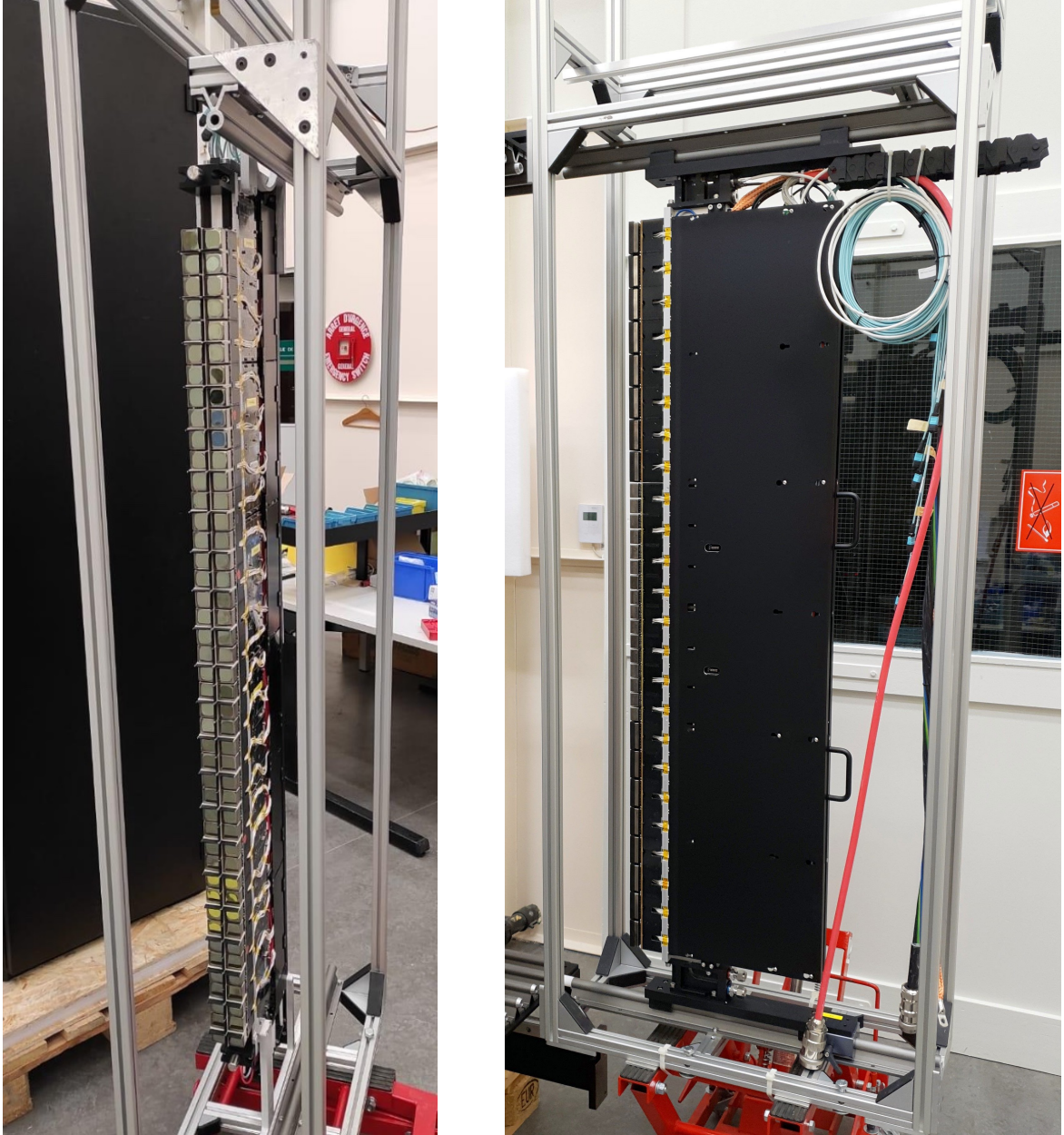
Figure 65. Pictures of (left) a completed RICH1 column (front view) and (right) a RICH2 column (side view, ECs on the left), with the photon detector chain and the complete set of services.
