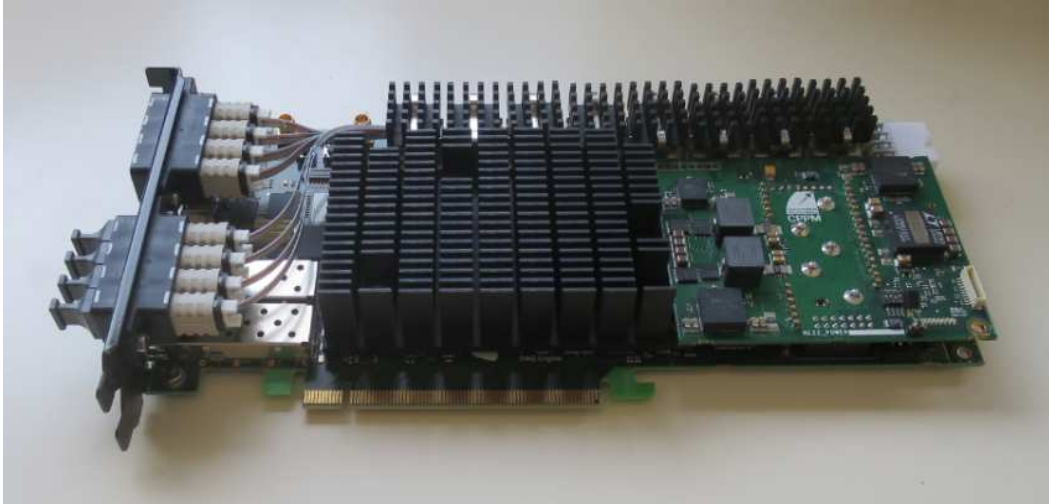
Figure 99. View of the PCIe40 board.
