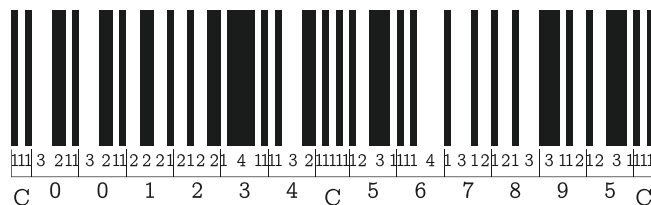
Fig. 4. Decoding the data stored in a UPC-A barcode. The top row of numbers shows the width of each bar. The bottom row shows the number encoded by each set of bars. Calibration bars are labeled C.
