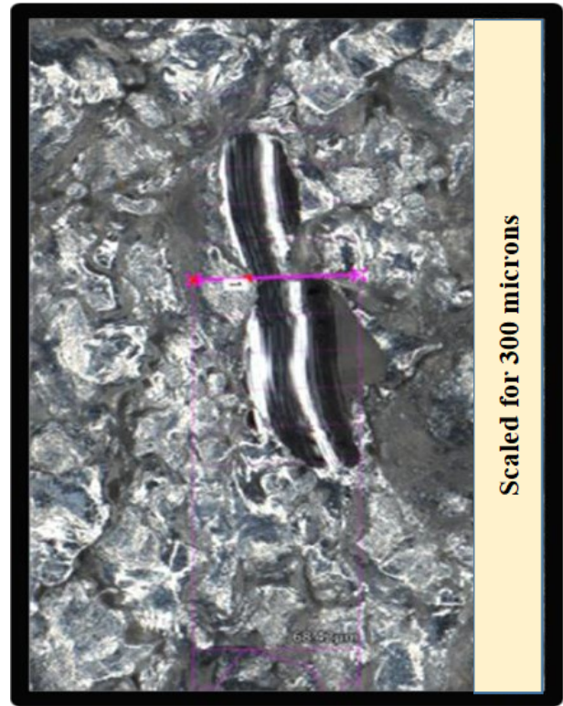
FIGURE 1: ILLUSTRATION OF A SCRATCH PERFORMED ON AN AM SAMPLE.
