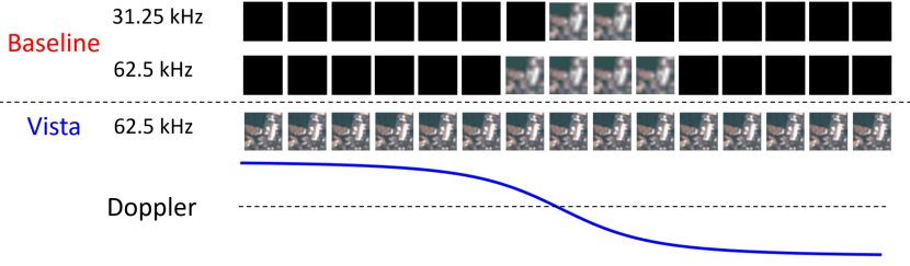
Fig. 13. Estimated image throughput over one pass of Vista CubeSat over an urban city with max elevation of 90^\circ and inclination angle of 97.52^\circ . Current terrestrial LoRa ground stations would be able to only detect and decode only 2–4 packets compared with the 15 encodings decoded via Vista.
