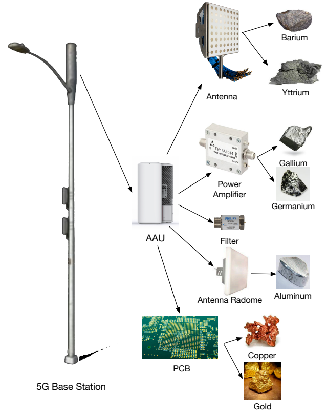
Fig. 1. 5G base station components and materials
