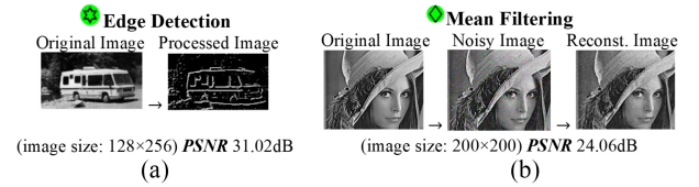
(image size: 128×256) PSNR 31.02dB (a) (image size: 200×200) PSNR 24.06dB (b) ● → N=256 , using circuit topology of [18], w/ optimized library, SLG, total P=10.56mW . ● → N=256 , using circuit topology of [20], w/ optimized library, SLG, total P=8.56mW , while w/o optimization P=11.67mW .
