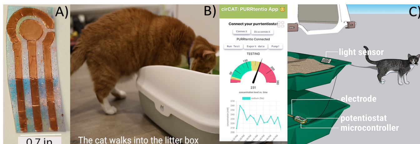
Figure 1: PURRtention a) DIY electrochemical biosensor b) Litter Box System and mobile application readouts. c) Components.
