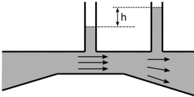
**Fig. 15.** Venturi effect, a change in velocity causes pressure difference in vertical tubes.
