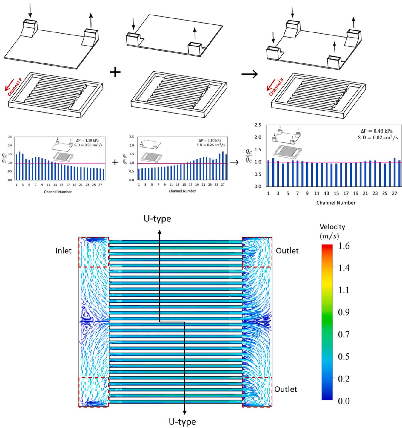
Fig. 33. Combination of two VU-type or two VN-type manifolds, flow distribution and pattern.
