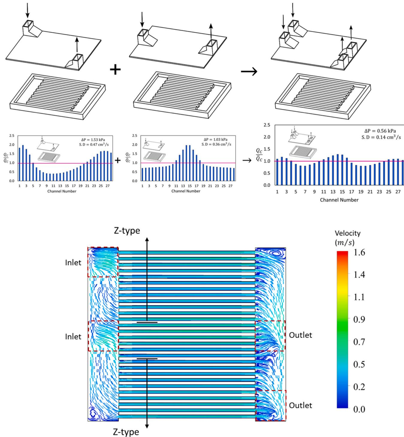
Fig. 29. Combination of VZ-type and VI-type manifolds, flow distribution and pattern.
