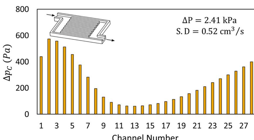
**Fig. 16.** Channel pressure drop for system with parallel Z-type manifold, channel pressure drop follows the same trend of channel flow rate.
