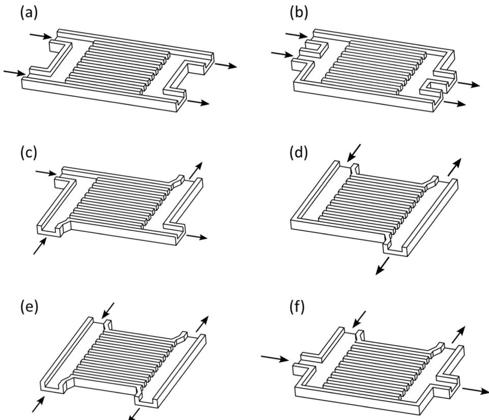
Fig. 9. The schematic of parallel combined manifold designs (a) Z+Z-type, (b) Z+I-type, (c) Z+N-type, (d) U+N-type, (e) U+U, and (f) U+I.
