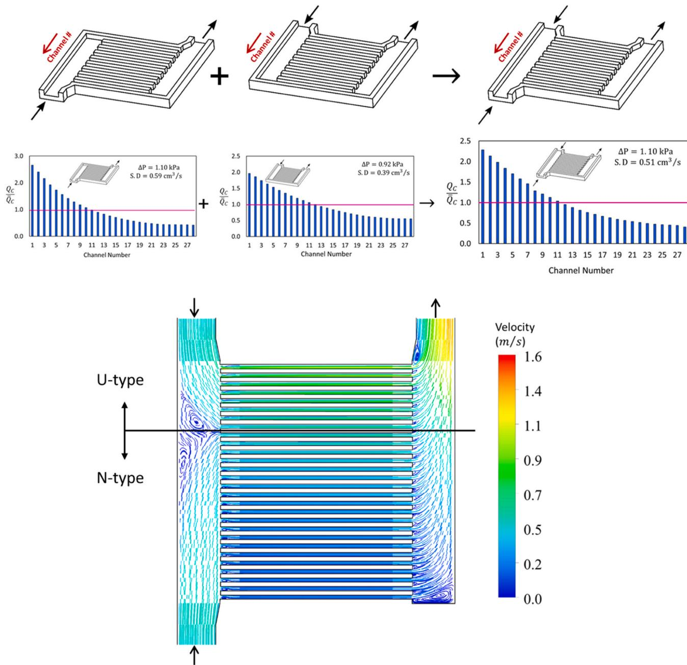
Fig. 19. Combination of N-type and U-type manifolds based on the same outlet, flow distribution and pattern.
