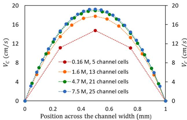
Fig. 4. Channel velocity profile for grids with different total and across-the-channel cells numbers.
