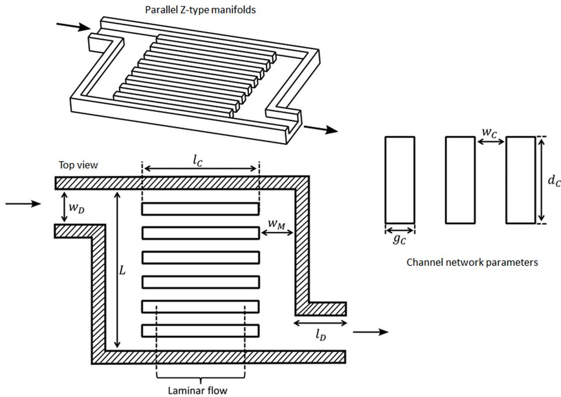
Fig. 2. Geometric parameters of the channel network-manifold system.
