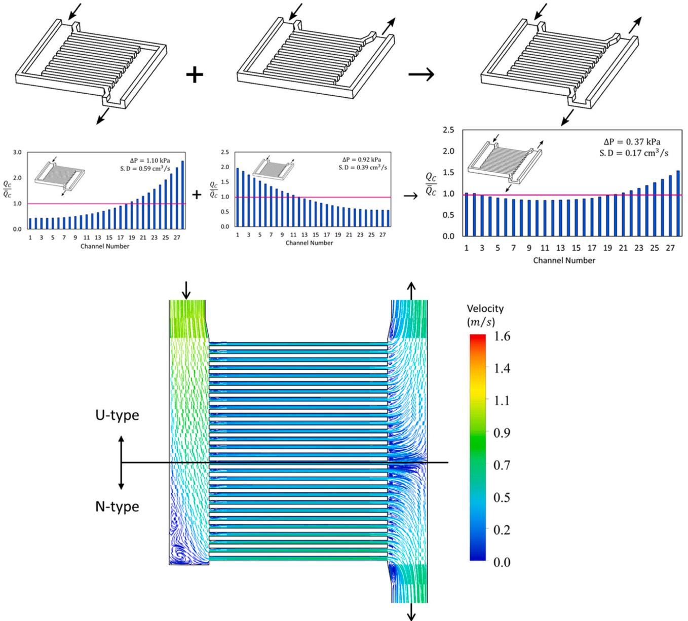
Fig. 18. Combination of N-type and U-type manifolds with a same inlet duct, flow distribution and pattern.
