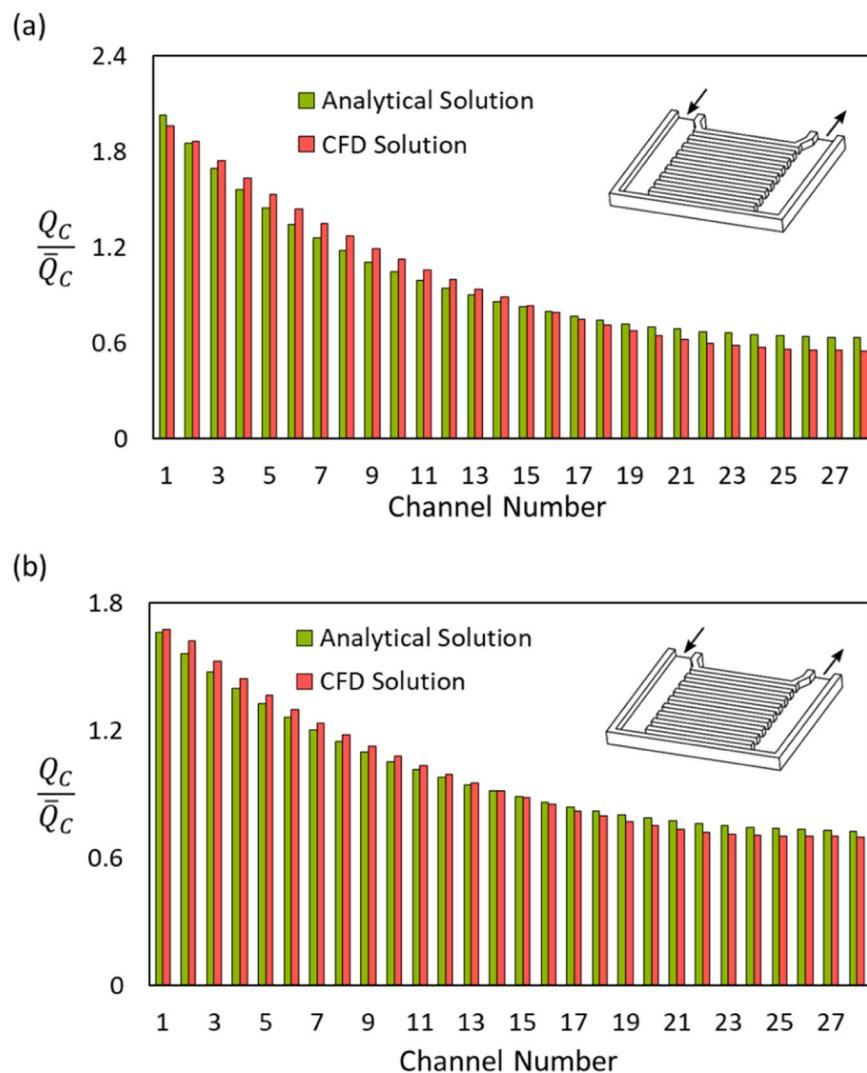
Fig. 7. Comparison of analytical and CFD solution for flow distribution through a U-type manifold system (a) at 1.5 LPM and (b) at 0.5 LPM total flow rate.
