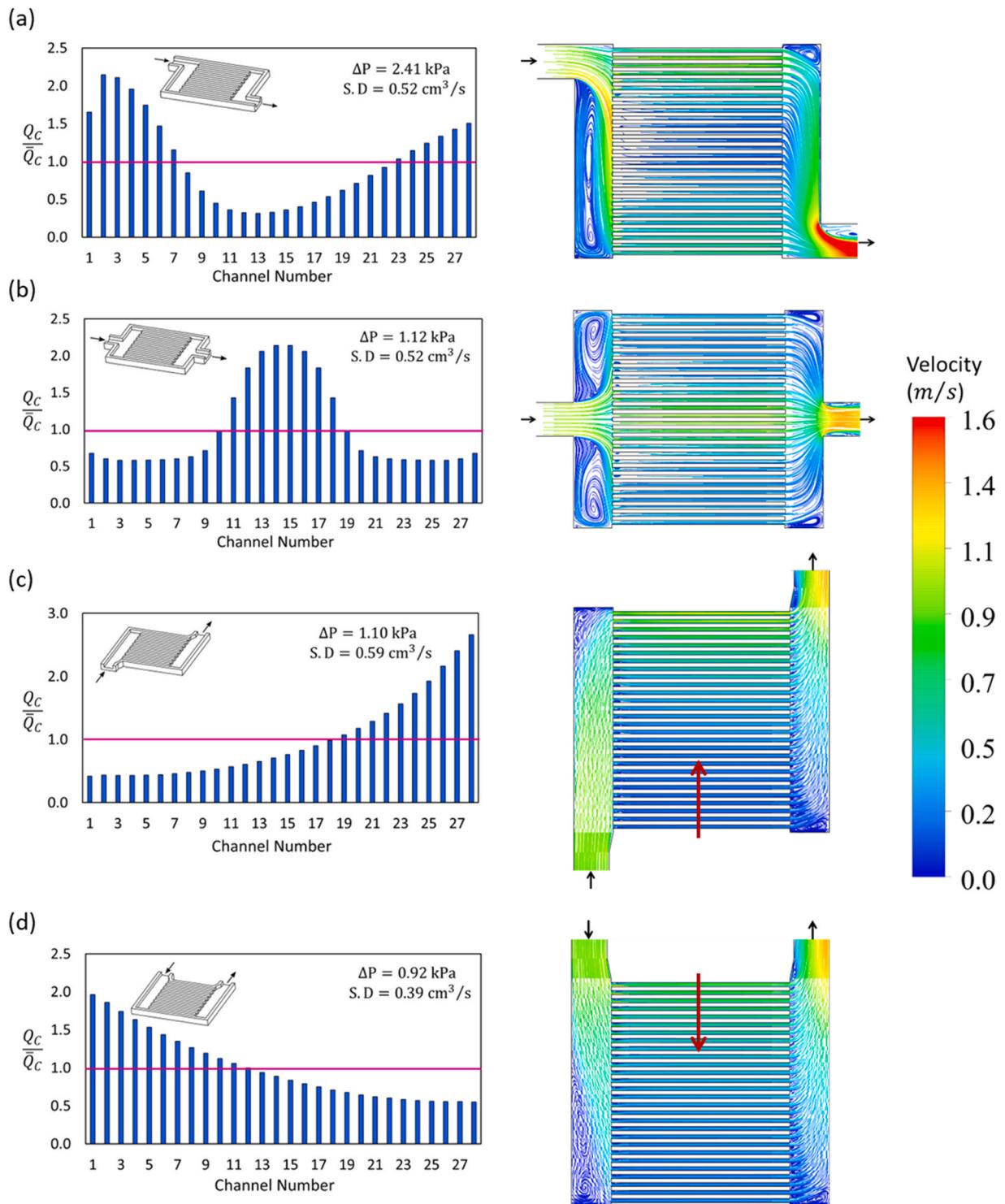
Fig. 14. Four parallel conventional manifold designs, flow distribution and pattern (a) Z-, (b) I-, (c) N-, and (d) U-type.
