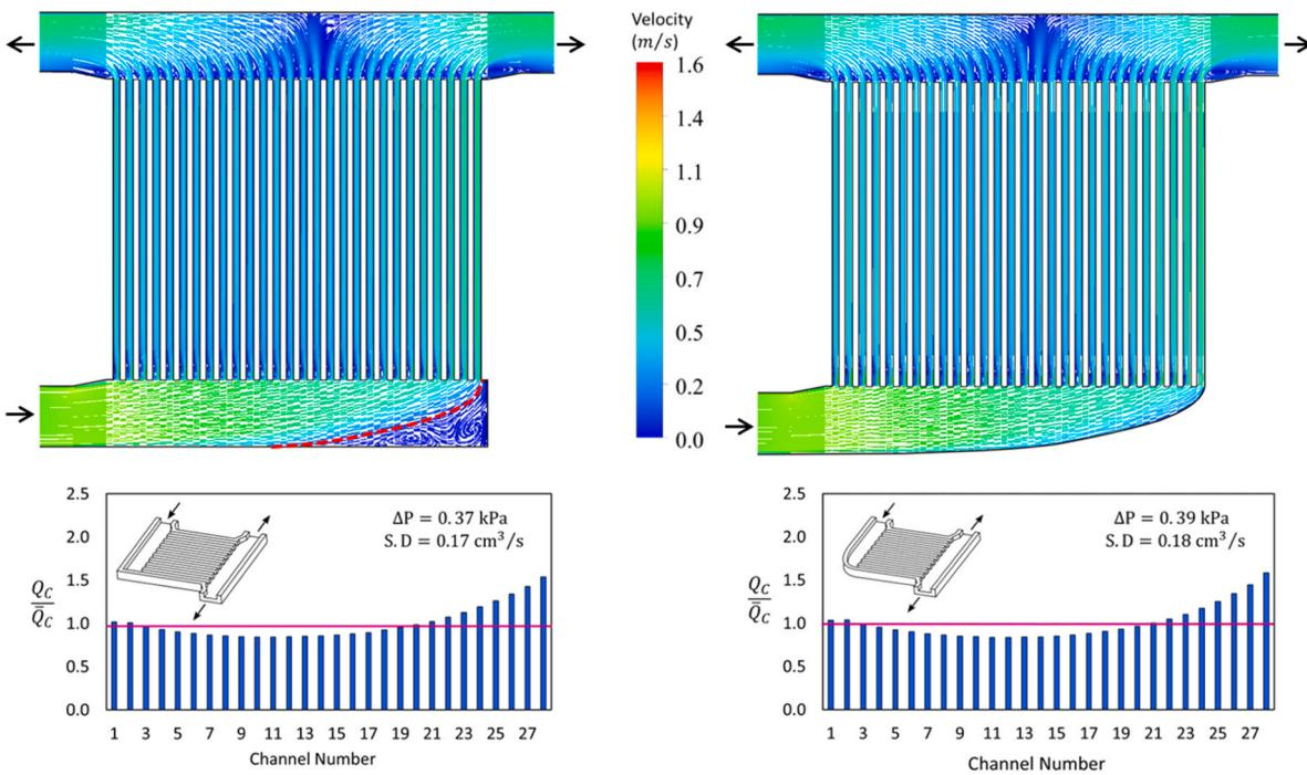
Fig. 25. Comparison of U+N type manifold and its streamlined version in flow distribution and pattern.
