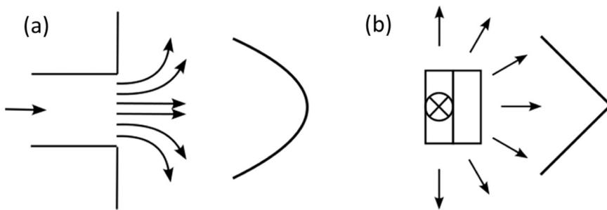
Fig. 27. (a) Flow distribution in middle channels of PI-type manifold and (b) VI-type manifold.
