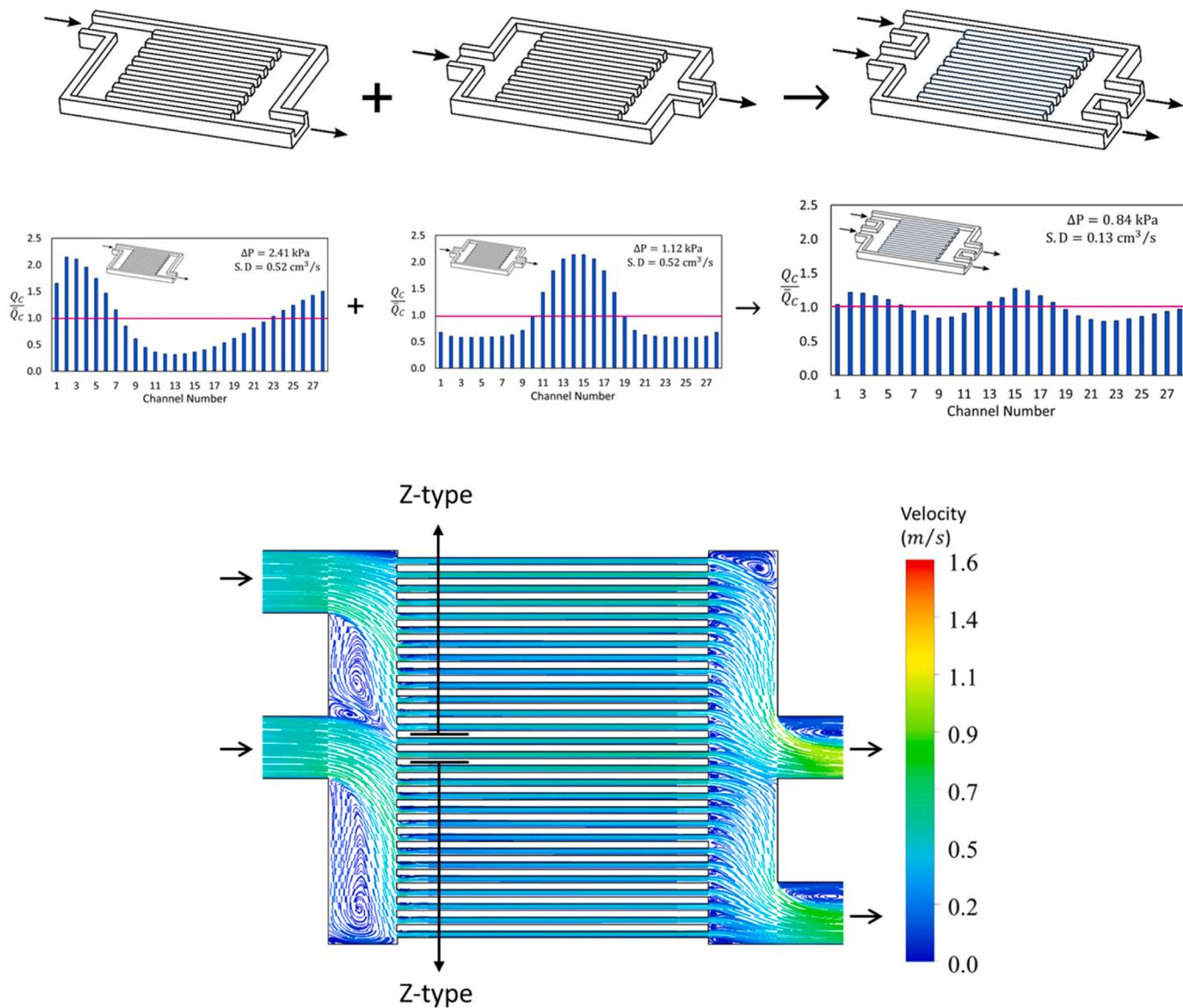
Fig. 20. Combination of Z-type and I-type manifolds, flow distribution and pattern.
