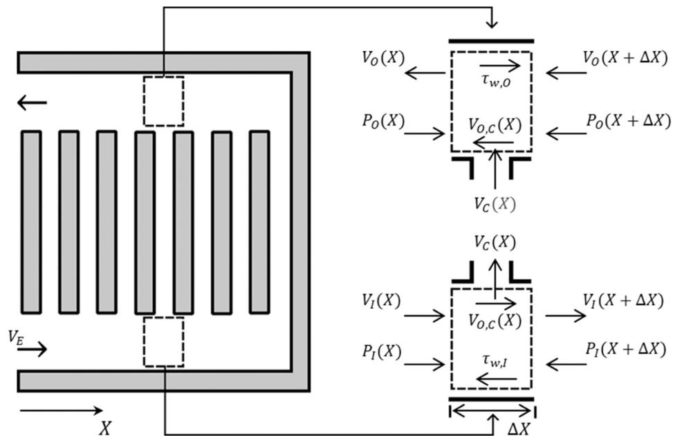
**Fig. 6.** Schematic of a U-type parallel channel system associated with control volumes in inlet and outlet manifolds used for developing the analytical model.
