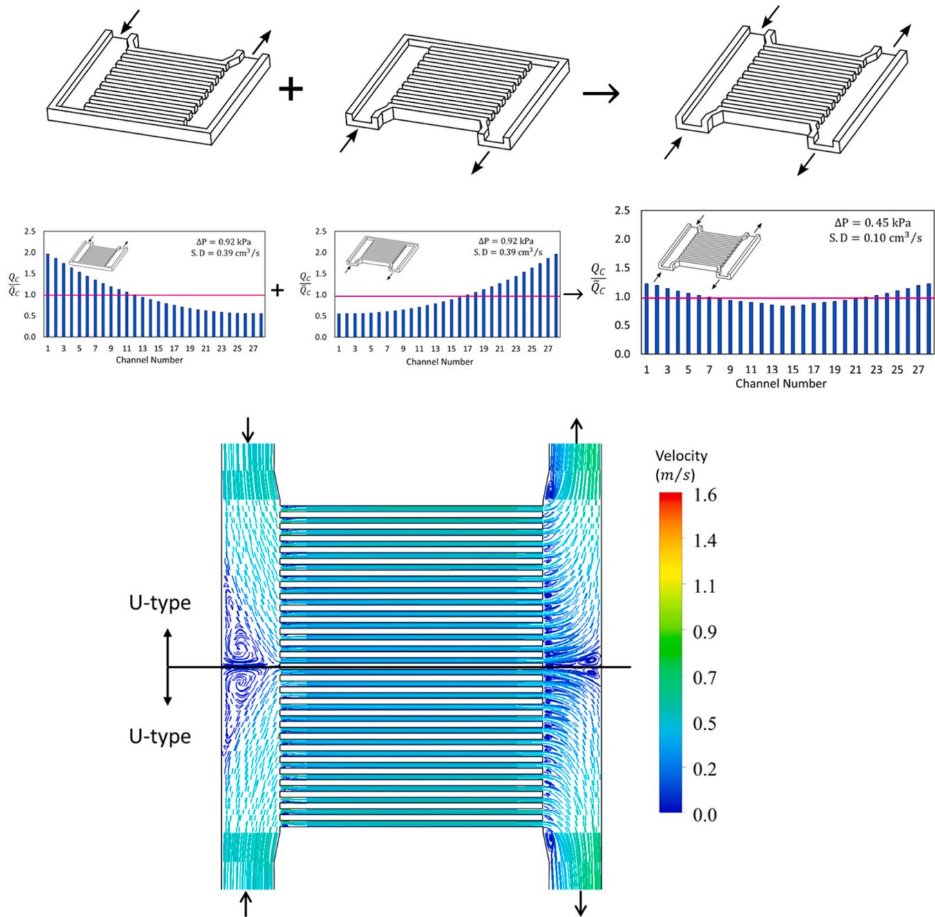
Fig. 23. Combination of two reflective U-type manifolds, flow distribution and pattern.
