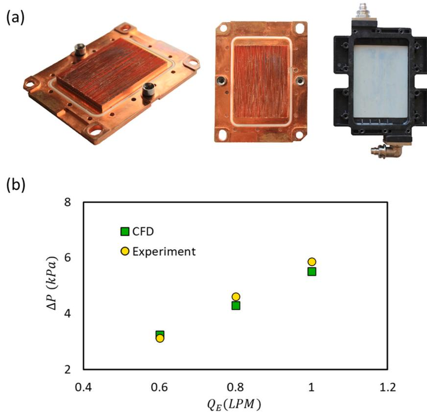
**Fig. 5.** Model methodology validation (a) the parallel channel water cooled heat sink with a Z-type manifold (b) comparison of numerical and experimental pressure drop data at three different flow rates.
