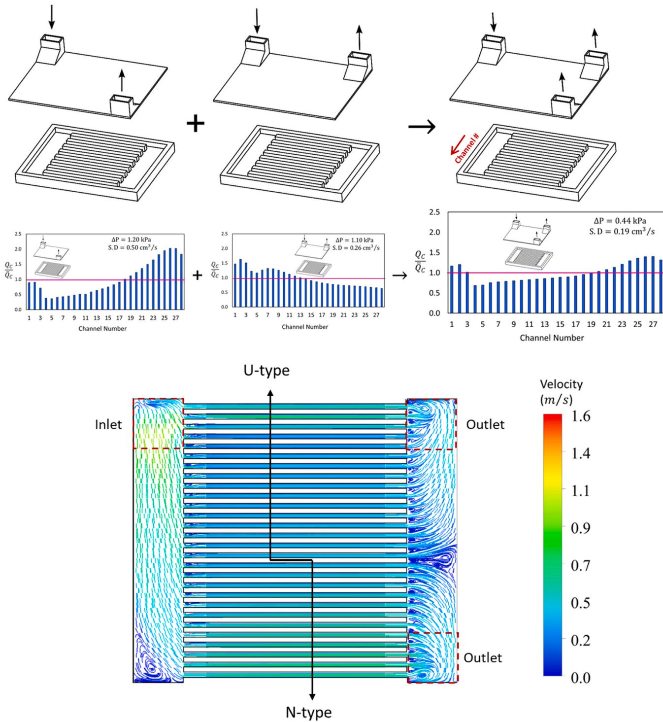
Fig. 28. Combination of VN-type and VU-type manifolds, flow distribution and pattern.
