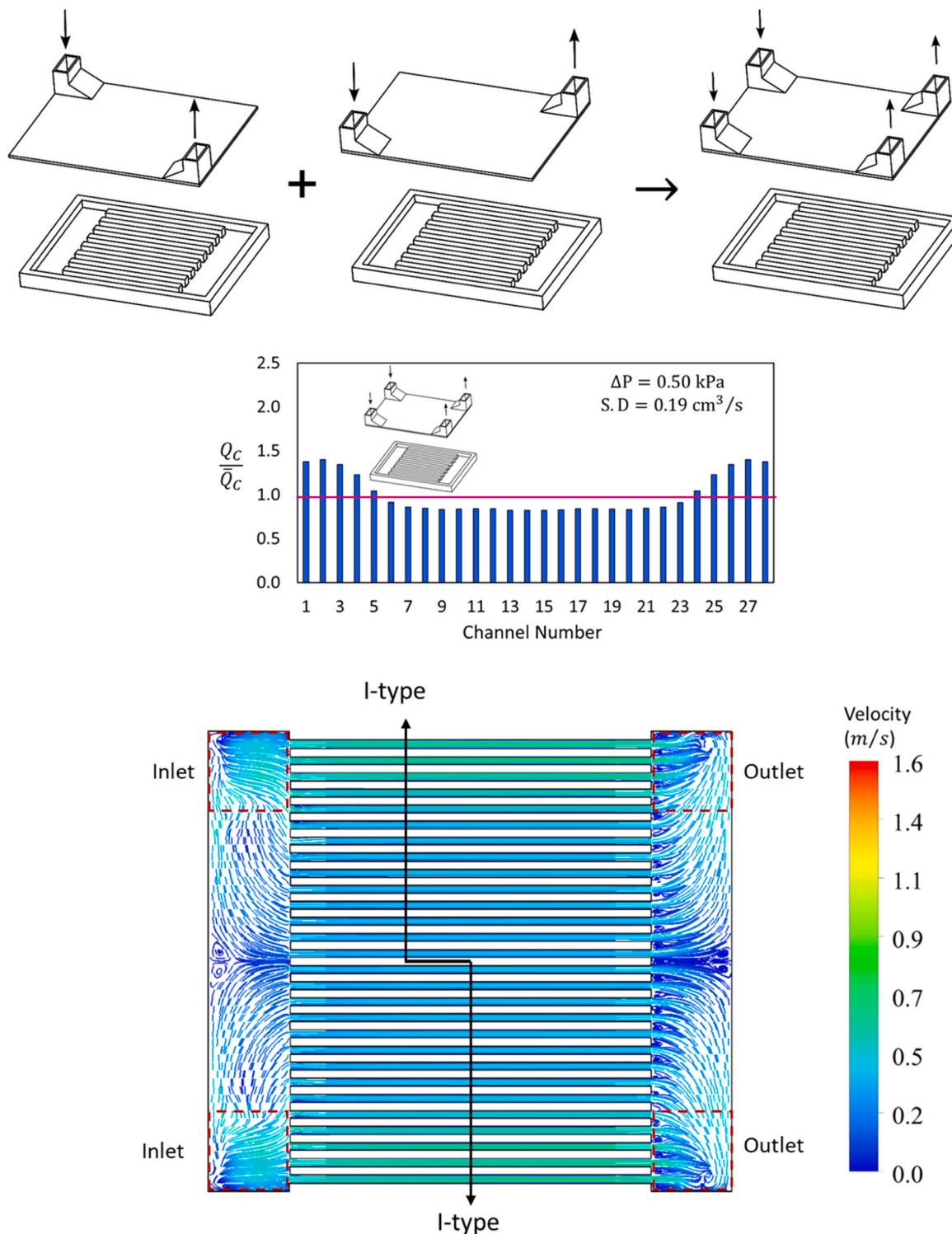
Fig. 30. Combination of two VZ-type manifolds, flow distribution and pattern.
