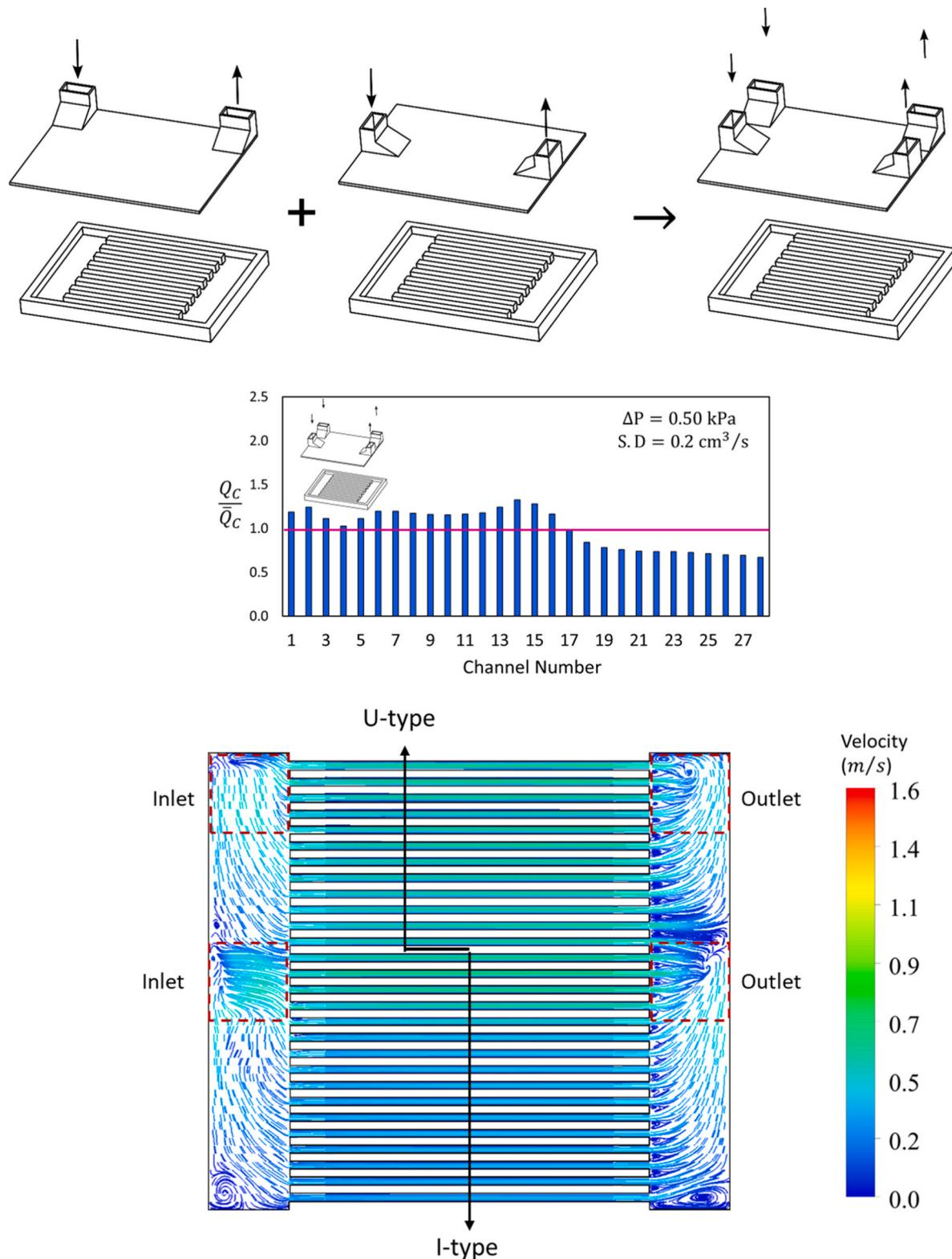
Fig. 32. Combination of VU-type and VI-type manifolds, flow distribution and pattern.
