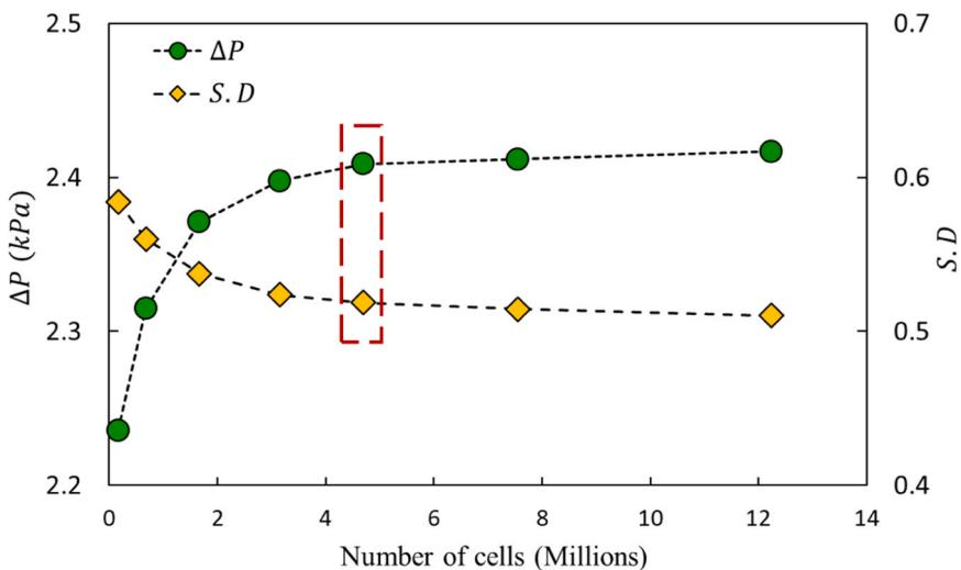
Fig. 3. The results of the discretization error analysis based on pressure drop and flow distribution standard deviation (the grid with 4.7 million cells is adopted).
