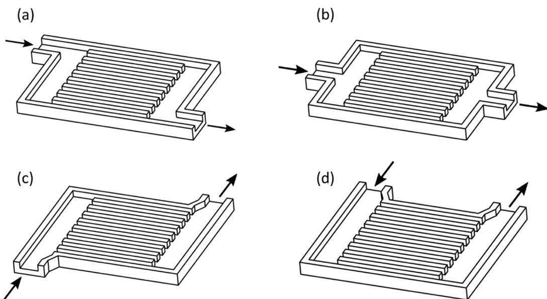
Fig. 8. The schematic of four basic common manifold designs (a) Z-type, (b) I-type, (c) N-type, and (d) U-type.
