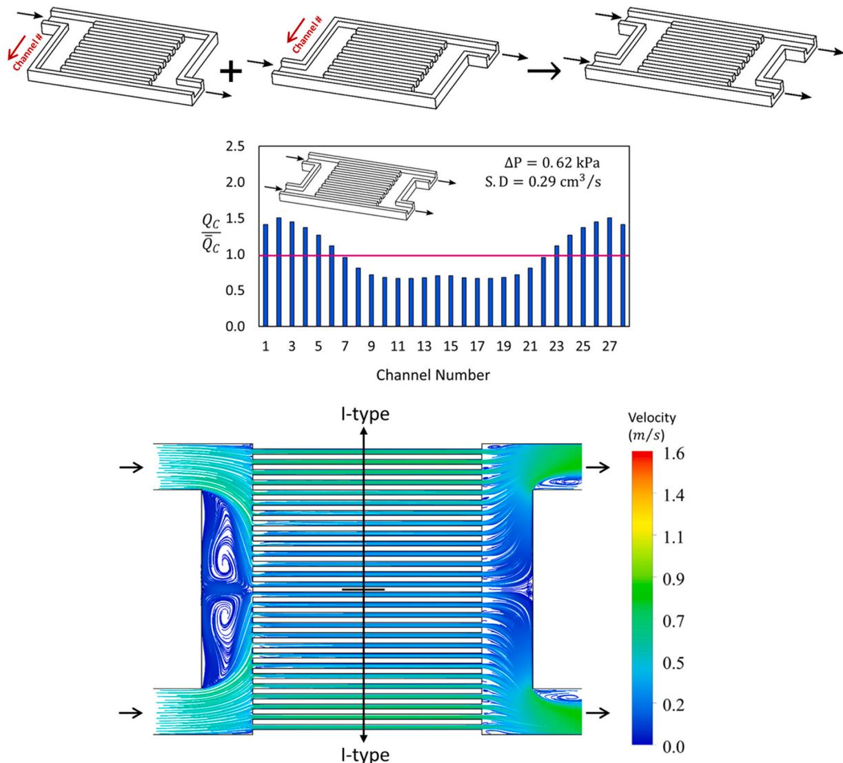
Fig. 21. Combination of two Z-type manifolds, flow distribution and pattern.
