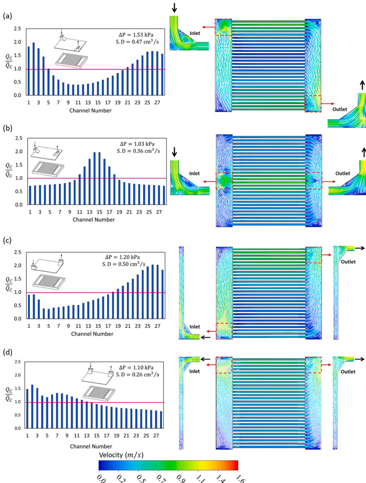
Fig. 26. Flow distribution and pattern for four basic vertical manifolds (a) VZ (b) VI (c) VN and (d) VU.
