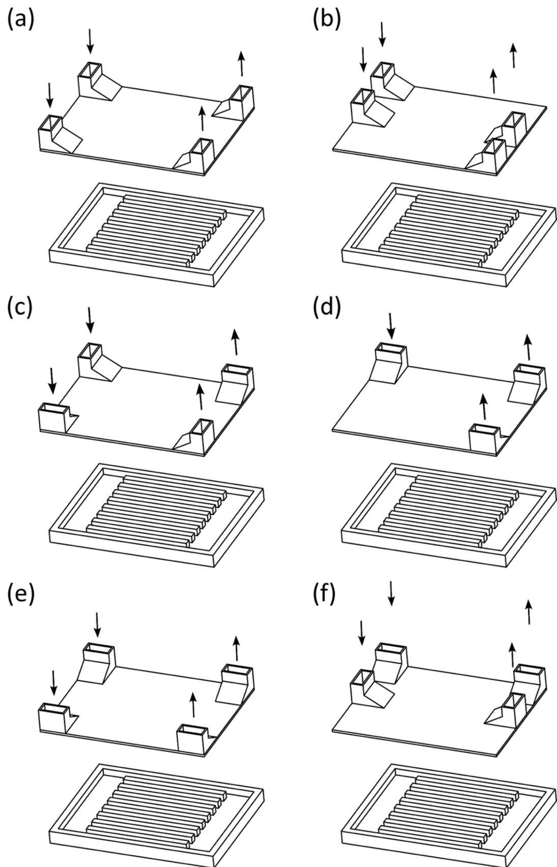
**Fig. 13.** The schematic of vertical combined manifold designs (a) VZ+VZ-type, (b) VZ+VI-type, (c) VZ+VN-type, (d) VU+VN-type, (e) VU+VU-type, and (f) VU+VI-type.
