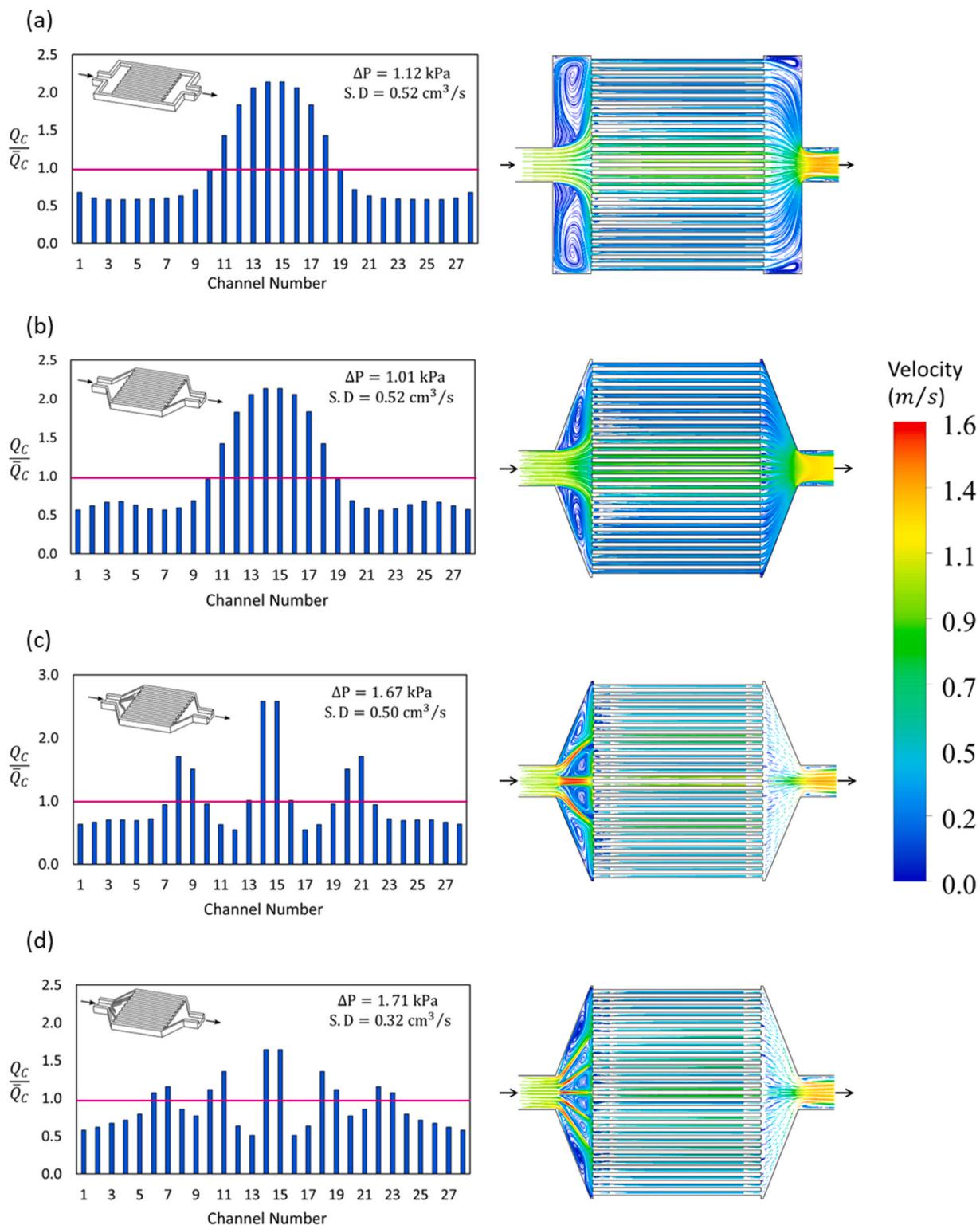
**Fig. 17.** Flow distribution and pattern in the class of the I-type manifold (a) original I-type, (b) diffuser-shaped, (c) diffuser-shaped with two guide vanes and (d) diffuser-shaped with four guide vanes.
