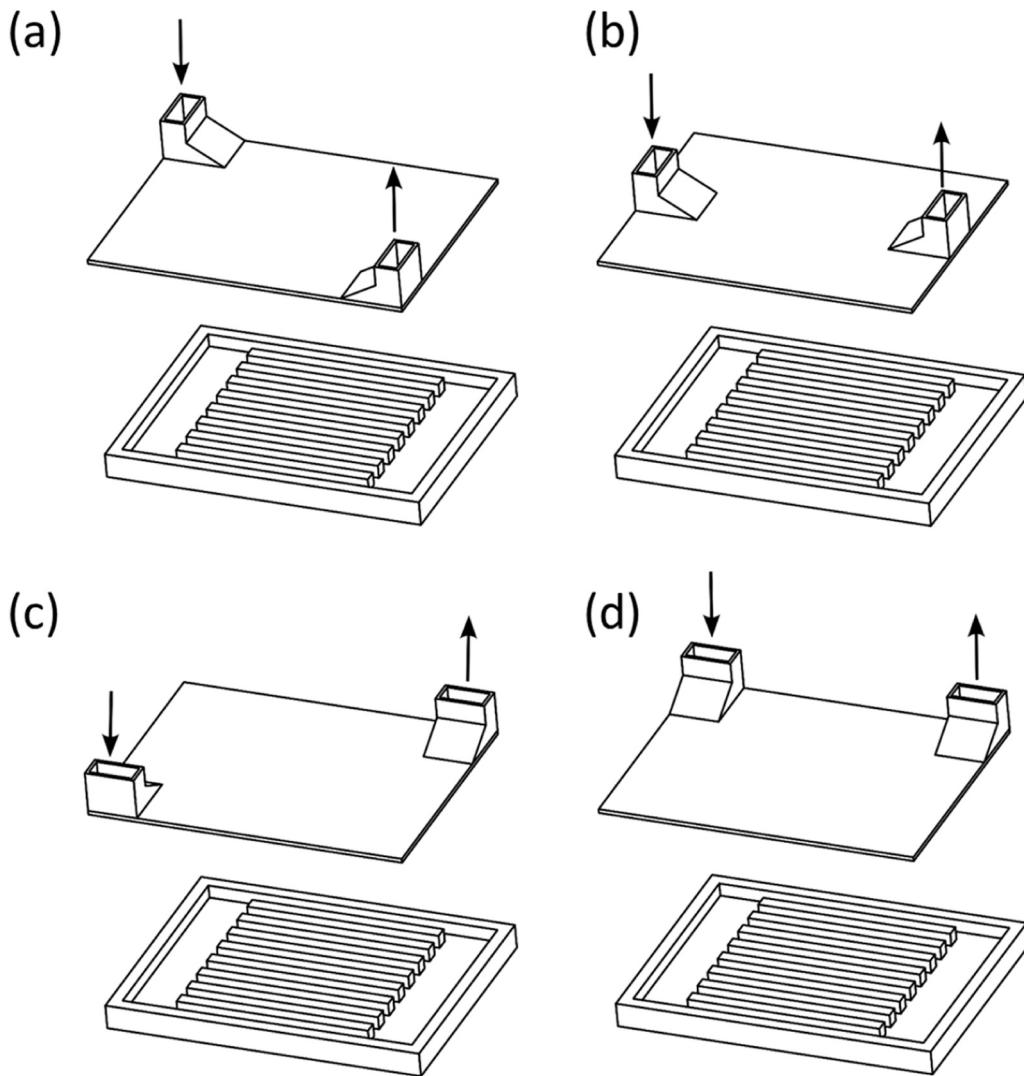
Fig. 12. The schematic of four basic vertical inlet-outlet manifold designs (a) VZ-type, (b) VI-type, (c) VN-type, and (d) VU-type.
