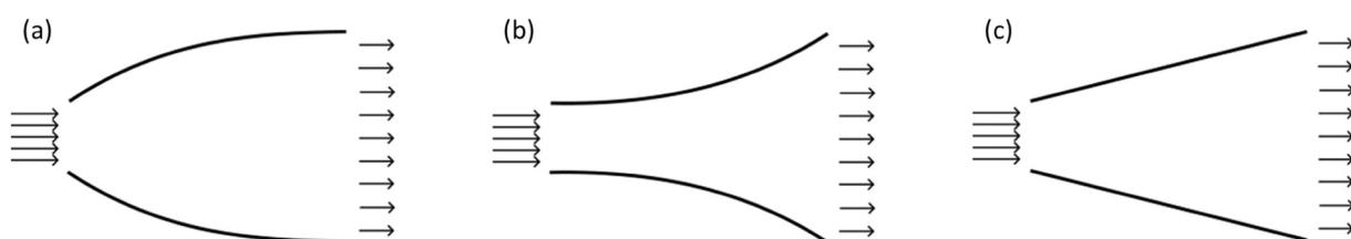
Fig. 11. Different shapes of diffuser (a) Bell shaped, (b) trumpet shaped, and (c) straight wall.
