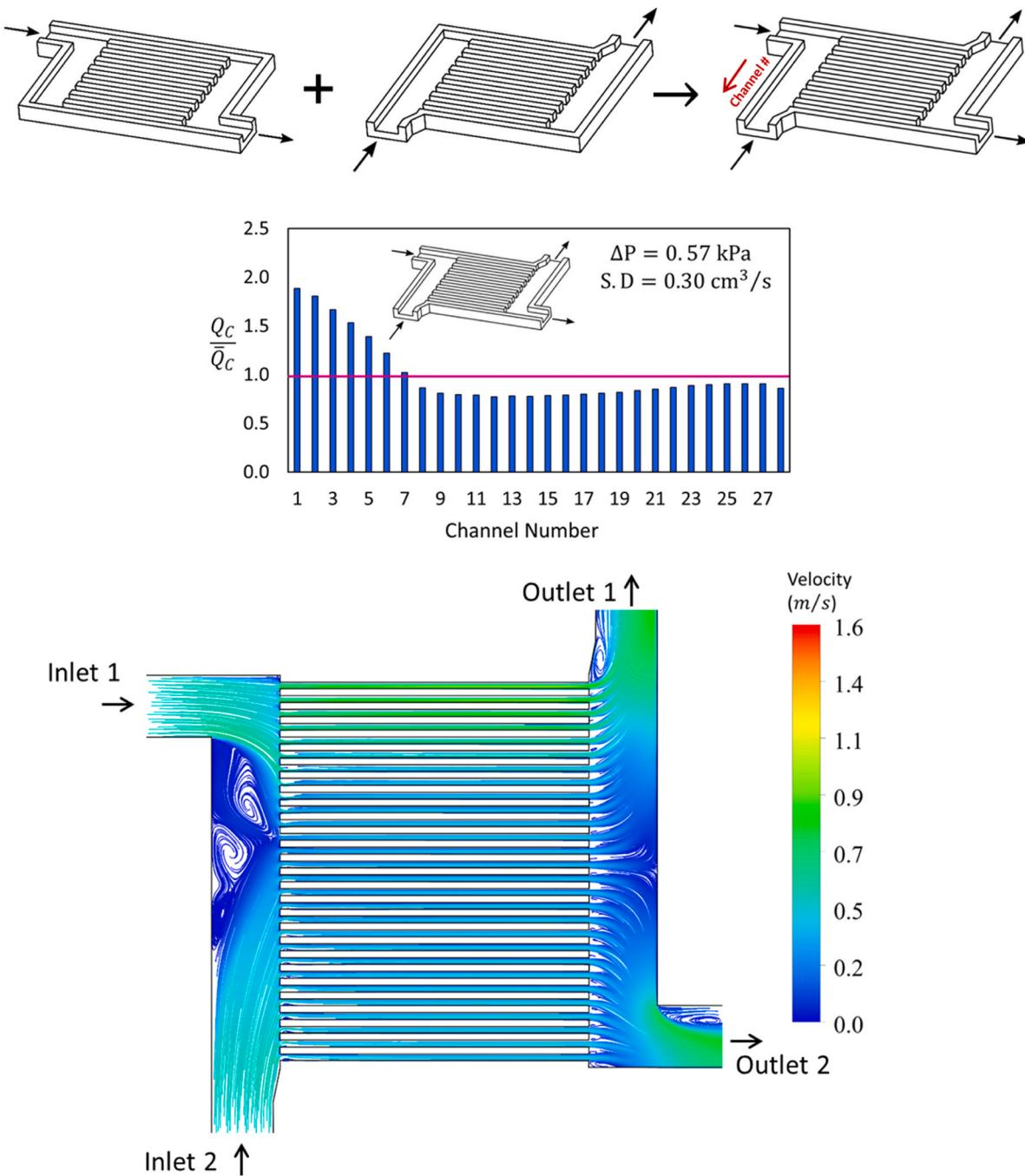
Fig. 22. Combination of Z-type and N-type manifolds, flow distribution and pattern.
