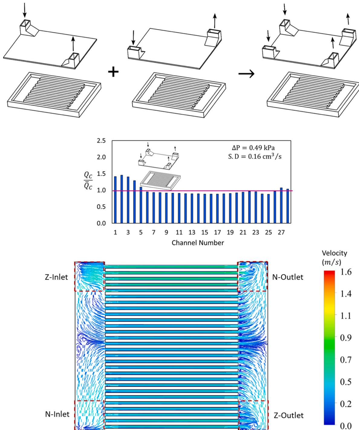
Fig. 31. Combination of VZ-type and VN-type manifolds, flow distribution and pattern.
