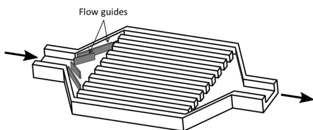
Fig. 10. Diffuser-Nozzle shaped manifolds with flow guides (blades).
