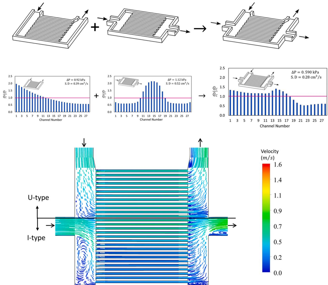
Fig. 24. Combination of U-type and I-type manifolds, flow distribution and pattern.
