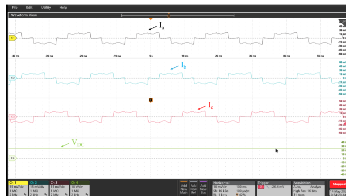
Figure 15. BLDC motor stator currents and DC-link voltage under healthy case at 1500 rpm.
