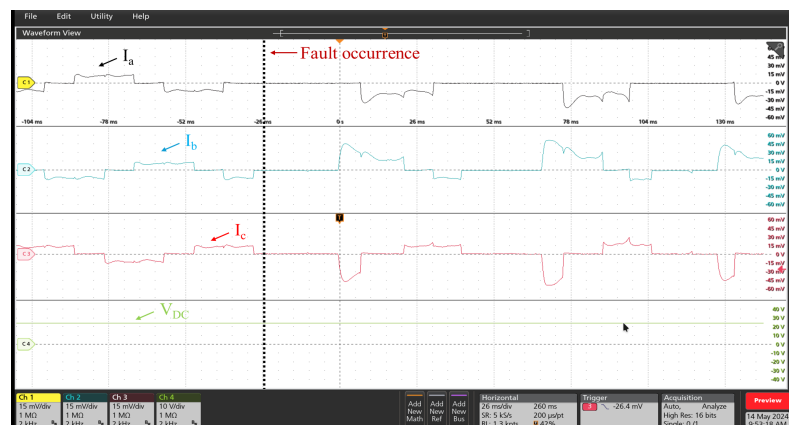
Figure 20. BLDC motor stator currents and DC-link voltage in the faulty case at 500 rpm.
