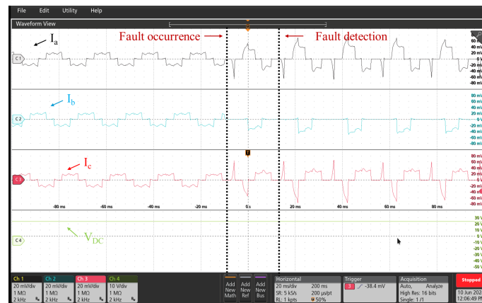
Figure 17. BLDC motor stator currents and DC-link voltage in the S_3 faulty case at 1500 rpm.
