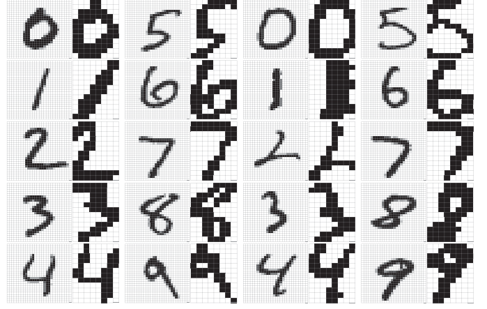
Fig. 3: Conversion of the MNIST handwritten digits from the original images ( 28 \times 28 gray color) to two-tone colored images ( 12 \times 8 binary color). The converted dataset is named TT-MNIST.
