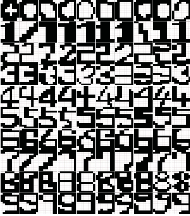
Fig. 2: Examples of user-generated digit patterns from the 2400-digit pattern dataset. Each pattern is created using the clickable pattern grid in the Neural Network Trainer system.
