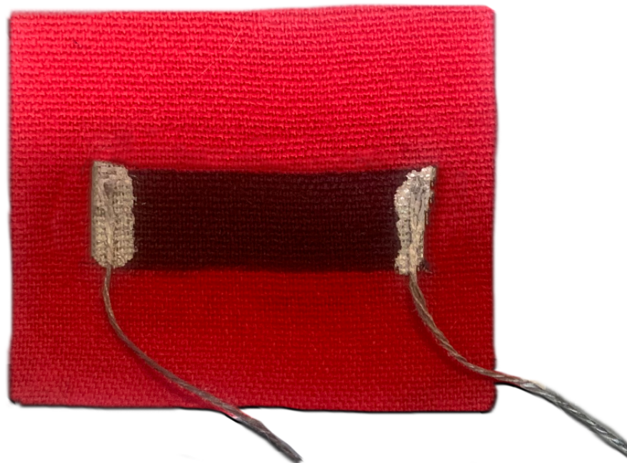
Figure 1. Motion Tape sample with conductive wire leads given to the physical therapists for evaluation.
