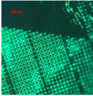
Figure 4. Fluorescence microscope image of patterned perovskite QDs after the blue backlight LED is turned on.
