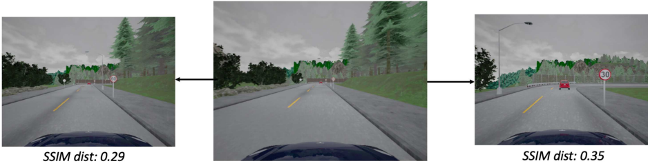
Fig. 2. SSIM distance illustration. Here we show an example of how SSIM distance works.
