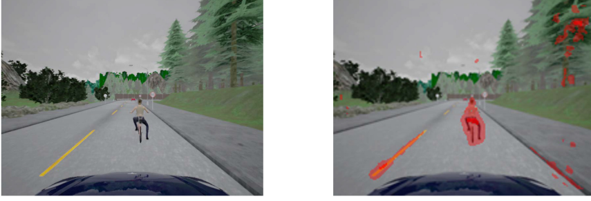
(a) Car does not detect the biker, leading to a crash (b) Frame detected as OOD; the region in red shows the pixels responsible for deviation
