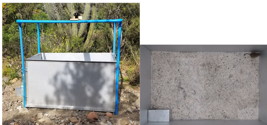
Figure A1. (Left) Open field box in situ with tetrapod (in blue) to hold video camera in place. (Right) Still image from video of behavioural trial. The box in the lower left corner of the OFB served as a hide for subjects, to which they acclimated for 3 min and, once opened, could return to for shelter.
