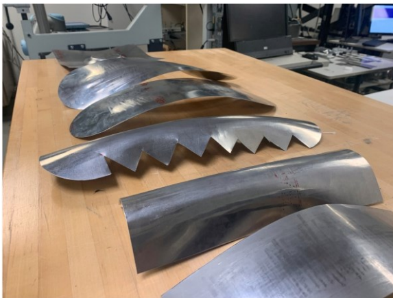
Fig. 2. High curvature panels manually formed with the English wheel. Fender-like objects are the desired target parts to show the capability of an integrated English wheeling system in the future. To make a complex piece like a fender through robotic forming, integrated components are essential.
