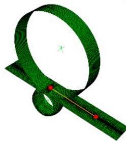
Fig. 8. (a) Key considerations when modeling single-track English wheeling: (1) definition of sheet engagement/compression, (2) mirroring the real-world kinematics or applying equivalent boundary conditions, and (3) choice of element type/meshing. (b) ABAQUS FEM models for single-track and multi-track wheeling. Equivalent model where displacement is prescribed on the wheels instead of on the sheet is used.
