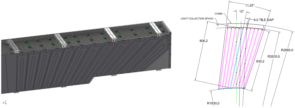
Fig. 5. Left: Scintillator tiles in a layer of the OHCal. Right: Transverse cutaway view of an OHCal module, showing the tilted tapered absorber plates. Light collection and cabling is on the outer radius at the top of the drawing.
