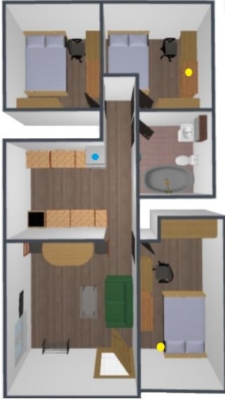
Figure 5: The layout of the apartment and locations of the tags. The yellow dots indicate BLE-AC models, while the blue dot inside the refrigerator is the UWB-Raw tag. The yellow dot closer to the right bottom corner is BLE-AC 1, while the other one on the top-right corner is BLE-AC 2.
