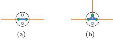
Figure 1: (a) A BSM measurement in the switch that fuses two quantum links by connecting two qubits. (b) A 3-GHZ measurement in a switch that fuses three quantum links by connecting three qubits. In both figures, the small blank circle in the switch denotes free qubits that are not entanglement, the small green circle in the switch denotes entangled qubits, the orange line indicates the quantum links to be fused, and the blue line shows the connection between qubits to fuse quantum links.
