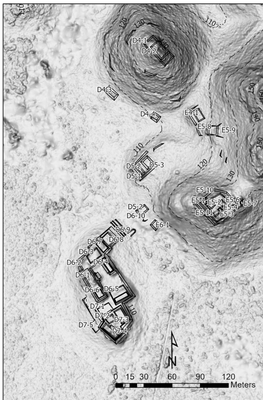
Figure 4. Multidirectional hillshade derived from 0.5 m resolution Lidar data showing architectural center of Budsilha with structures labeled; 10 m contour intervals indicate meters above sea level. Image by Charles Golden, PABC.
