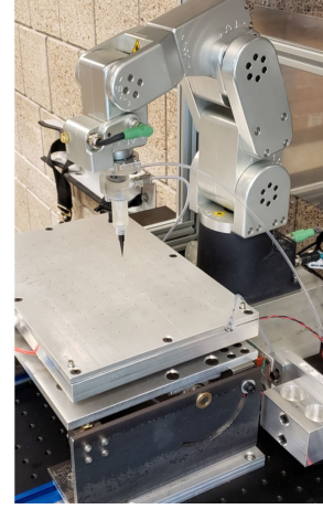
Fig. 6. Robotic arm with six degrees of freedom.
