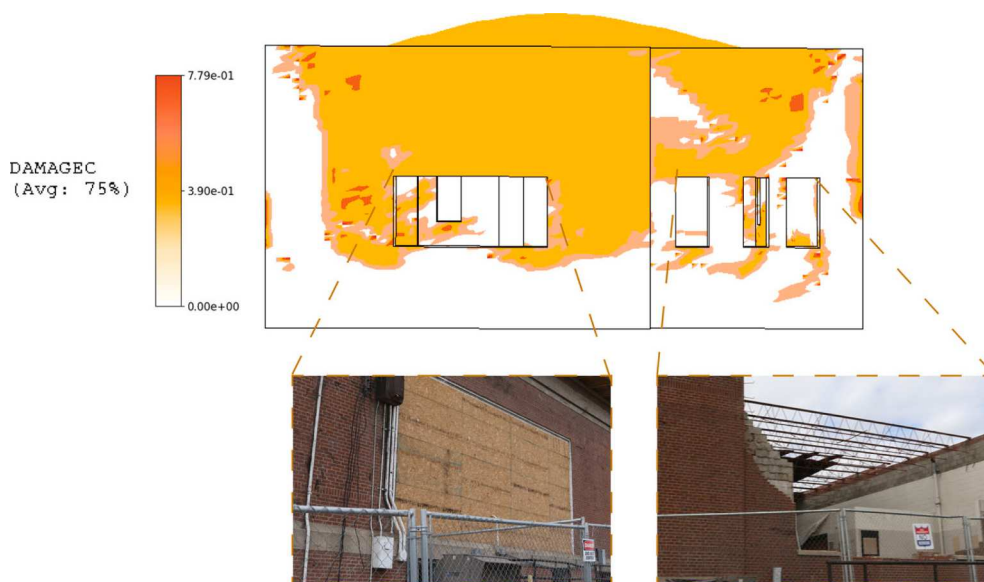
Fig. 7. Comparison between the nonlinear static analysis and the damage seen on-site.
