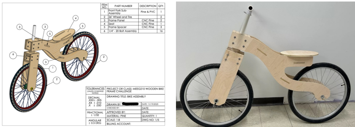
Figure 2. Example student work for final bike frame design: CAD assembly drawing (left) and assembled prototype (right).
