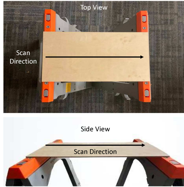
Fig. 1. Annotated photographs of our laboratory test apparatus with a plywood material sample. Material samples were placed between two plastic sawhorses, and GPR traces were taken in the scan direction indicated in the figure. Note the arrow represents the movement of the device, with signals being emitted perpendicular to this arrow (i.e., towards the floor).
