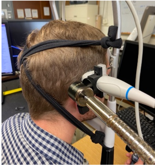
Fig. 1. The head rig is shown with a subject in place. The chin and forehead are placed in rests and cloth straps hold the head in place to minimize motion. The transducer is also held fixed relative to the rig using a custom fixation device.
