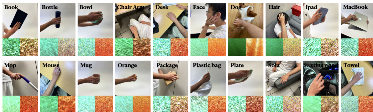
Fig. 1. Our hands engage with a wide variety of objects. These objects are often in contact with the fingers, which makes for an ideal location for sensor instrumentation. TextureSight implements wearable laser speckle imaging to distinguish between surface profiles (i.e., textures) for object recognition, which serves as a strong context clue for higher-order activity recognition.
