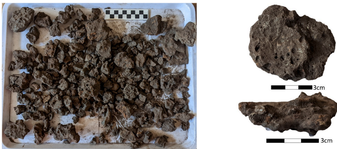
Fig. 4. Smithing slags from Unit 1, context [003], directly above [006]. (Left) a 50% subsample of excavated slags. With the exception of several complete and partial planoconvex smithing slags, the vast majority by volume are \leq 2 cm in diameter and broken, indicating manual breaking up of slags during smithing. (Right) two characteristic plano-convex smithing hearth slags from the same context. (For interpretation of the references to color in this figure legend, the reader is referred to the Web version of this article.)
