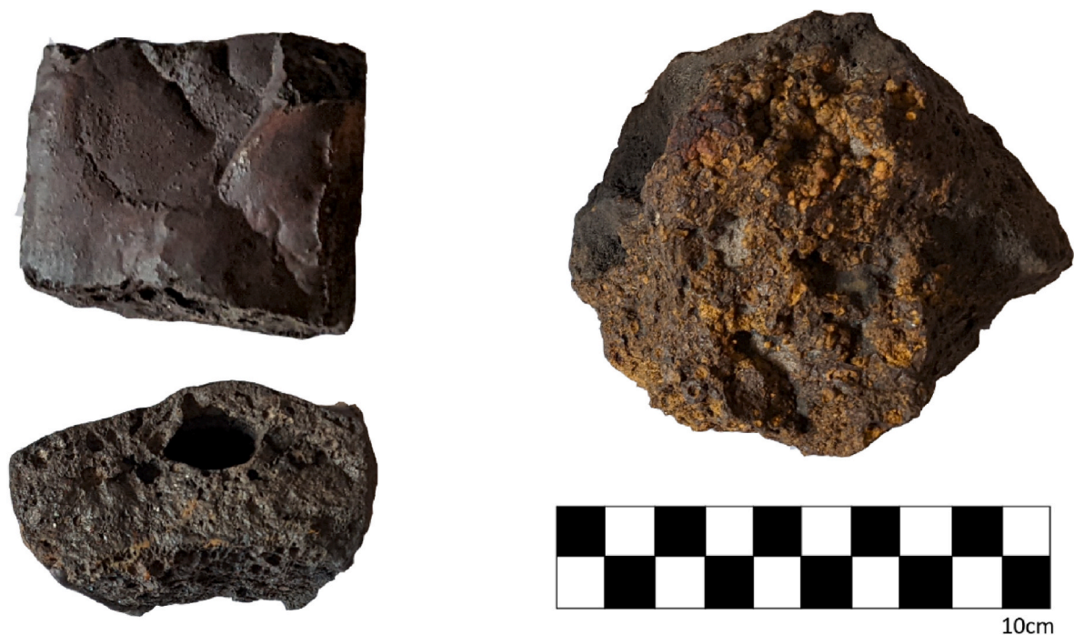
Fig. 6. Smelting debris from A4. (Left) top and side view of tuyere-tapped slag. (Right) large piece of ferricrete ore. (For interpretation of the references to color in this figure legend, the reader is referred to the Web version of this article.)
