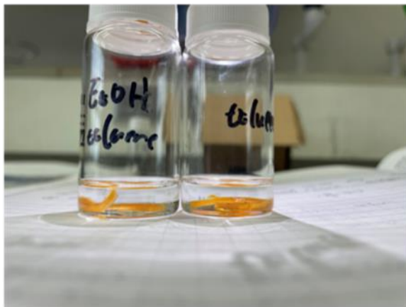
Figure S18. Pictures of vials with polymer network specimens in solvents (6 mL) before (A) and after (B) being heated at 80 °C for 24 h (left vial: in ethanol/toluene 1/2 v/v; right vial: in toluene).
