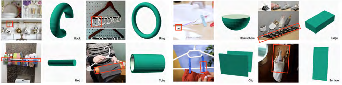
Figure 2: We analyzed 24 rigid undeformed fixture hacks and extracted eight connector primitive types found on objects in those hacks; Table 4 in Appendix A documents the shape parameters we use to parametrize a primitive’s geometry. We show each connector next to an example hack where it appears. The eight example hacks (left to right, top to bottom) are cup hanger (No.24), scarf organizer (No.22), toothbrush holder (No.7), charger holder (No.18), bathroom organizer (No.11), nonslip hanger (No.3), pants hanger (No.8), and soap bottle bag (No.1) as numbered in Table 2 in Appendix A.
