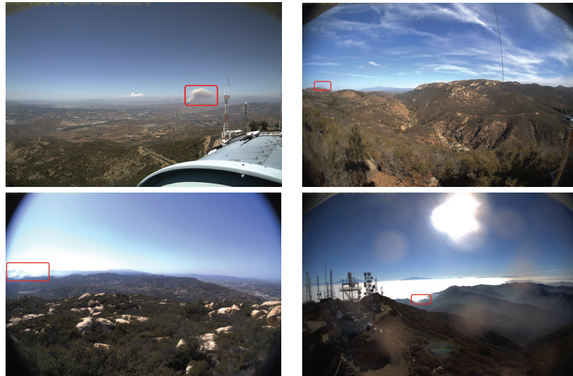
Figure 1. Sample images with smoke from the FlgLib dataset. The red bounding box indicates the location of the smoke plume. ( Top left ) Very apparent smoke plume; ( top right ) extremely faint smoke observed at a distance from the camera; ( bottom Left ) smoke blending into the area with strong glare; ( bottom right ) smoke with misleading haze.
