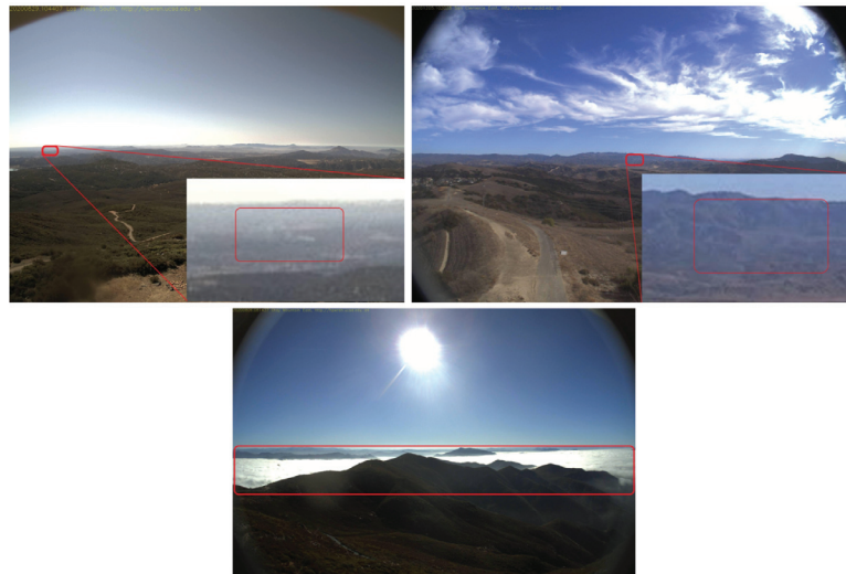
Figure 5. Qualitative results from baseline SmokeyNet and Multimodal SmokeyNet. ( Top left ) The red BB indicates the location of the smoke plume in the distance; TTD for mSN was found to be much smaller than that for SN. ( Top right ) The red BB encloses a very faint smoke plume in the image, which mSN correctly detected. ( Bottom row ) The area enclosed by the red BB shows a cover of low-hanging clouds; both SN and mSN incorrectly classified this image as containing smoke. Abbr.: BB = bounding box; SN = Baseline SmokeyNet; mSN = Multimodal SmokeyNet; TTD = time-to-detect.
