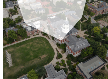
Fig. 2: A binary mask overlaid on an input image for visualization. The mask is generated by an intersection test with rays cast from each pixel and a bounding box. Rays that do not intersect with the bounding box are excluded, allowing a focused and shorter training process.
