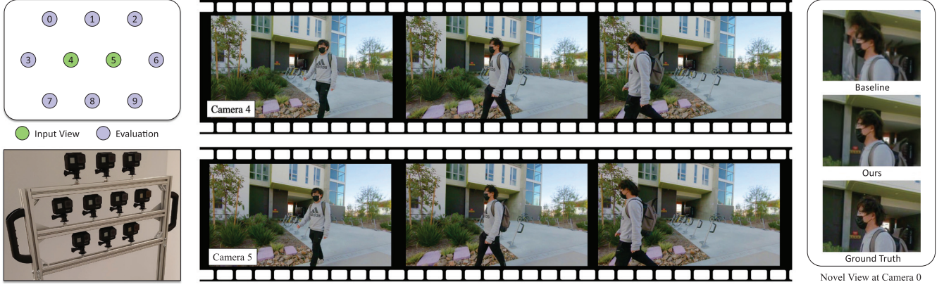
Fig. 1. Our custom camera rig. Top left figure shows the configuration we use for evaluation in Section V. We show the input stereo image sequences from camera 4 and camera 5 in the middle. The rightmost column shows the crops of rendered novel view at camera 0. Artifacts appear when the novel view is translated by a larger distance. We use the conventional MPI method [1] as our baseline algorithm. Note how the area on top of the person’s head is distorted and shows “stack of cards” artifacts. This type of artifact flickers in a dynamic video as the network hallucinates the disocclusion per-frame.
