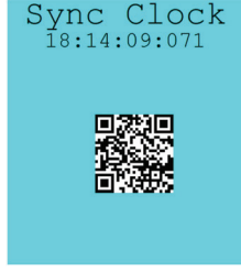
Fig. 2. Digital clock and the randomly moving QR code pattern used to perform synchronization. We have two ways to do synchronization: (1) matching the timestamp; (2) aligning the QR code location in all views. We use these methods to ensure the synchronization is accurate enough.
