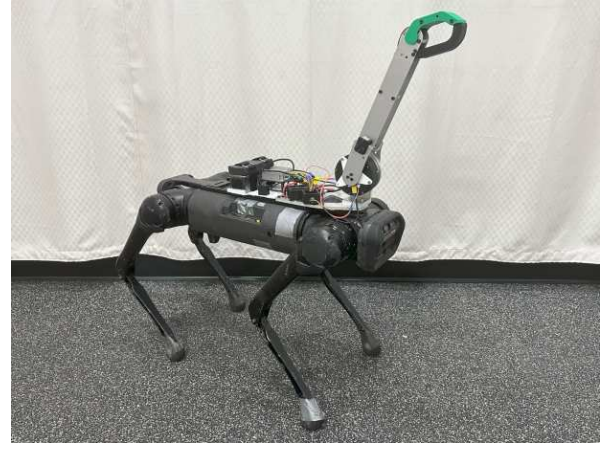
Fig. 3: Unitree Aliengo with custom-made arm used for experimental validation of the proposed approach
