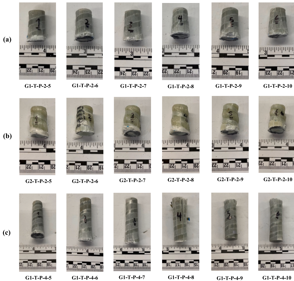
Fig. 8. Specimens after compressive test.
