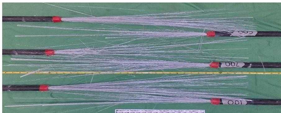
Fig. 7. Typical failure of GFRP bars after tensile test.
