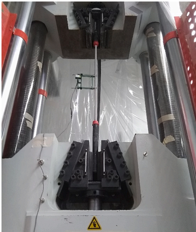
Fig. 4. Tensile test setup according to ASTM D7205.
