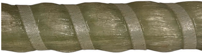
Fig. 11. Surface profile of G2 bar.
